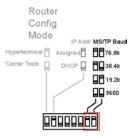
MS/TP Station ID - Defines the MS/TP MAC address of the i-Vu® Link/Open Link on the MS/TP network.
