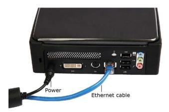
3 If you are using the USB Open Adapter to connect to an MS/TP network, plug the adapter into the USB port and connect to your network.
