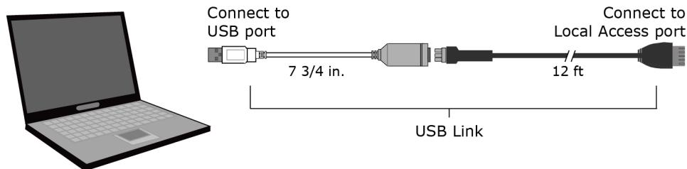
**NOTE** If using a USB isolator, plug the isolator into your computer's USB port, and then plug the USB Link into the isolator.
