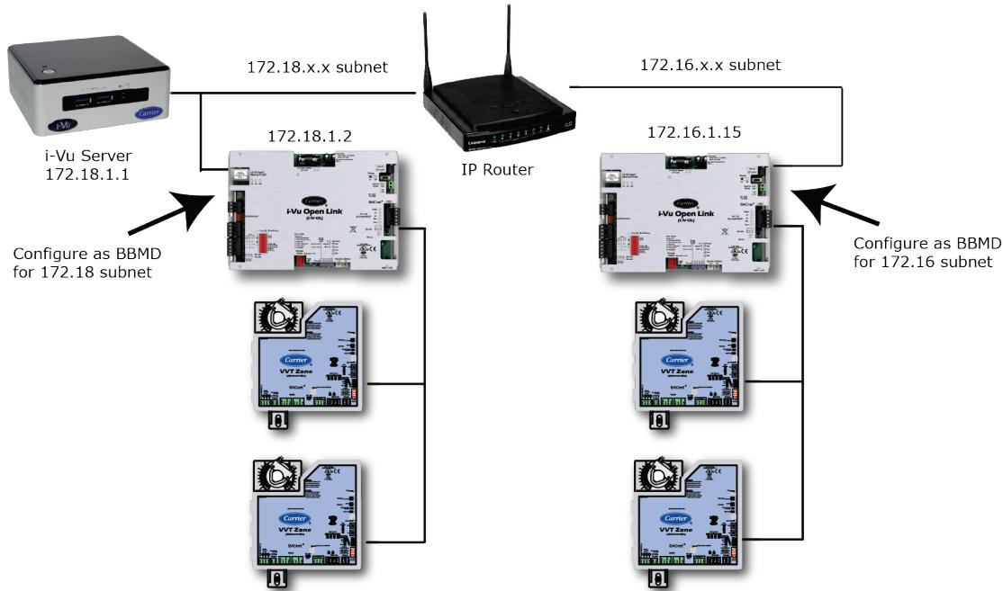
If your system has multiple routers that reside on different IP subnets, you must set up one router on each IP subnet as a BACnet/IP Broadcast Management Device (BBMD).
