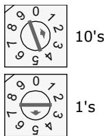
**CAUTION** The factory default setting is **00** and must be changed to successfully install your UC Open.
