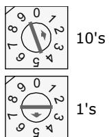
**CAUTION** The factory default setting is **00** and must be changed to successfully install your UPC Open.
