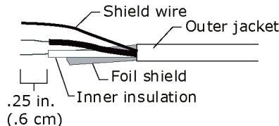
**3** Strip about .25 inch (.6 cm) of the inner insulation from each wire.
