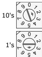
**NOTE** The Fan Coil recognizes its address only after power has been cycled.
