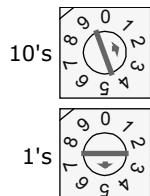
**NOTE** The Fan Coil recognizes its address only after power has been cycled.
