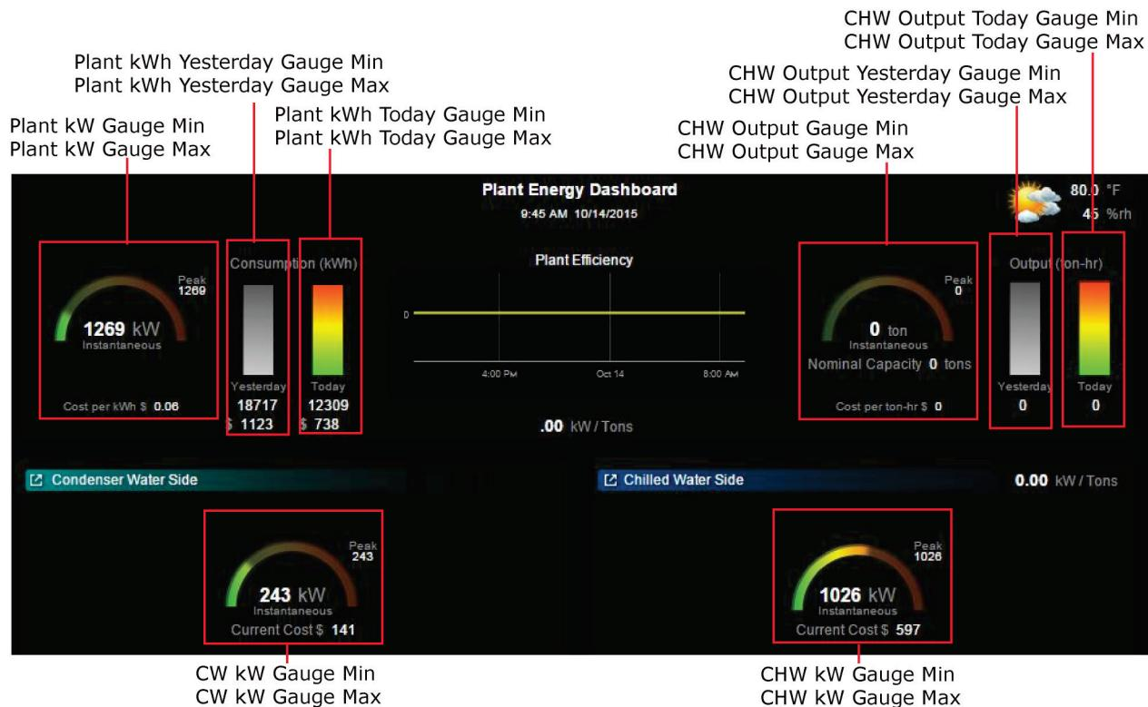
Enter cost value and set up gauges
