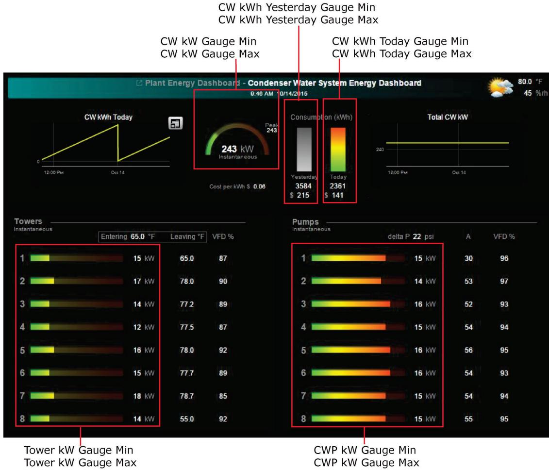
Enter cost value and set up gauges
