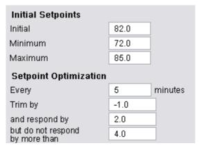
If the microblock outputs 75° and 5 minutes later the **req** input sees 2 requests, the new setpoint is  $78^{\circ} = 75 + (-1) + (2 \times 2.0)$
