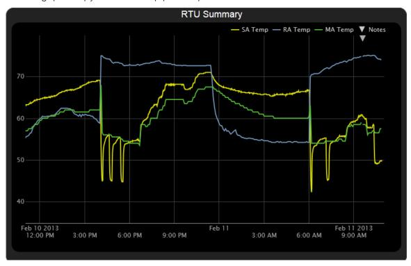
You can collect trend data for any point value in the Field Assistant system. The controller reads point values at intervals that you define and then stores that data in the controller. A controller has limited memory for storing trend data.
