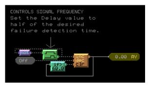
The logic in the network input's control program that receives the changing value. The SIGNAL analog network input's **Address** field contains the address of the BACnet Analog Value microblock sending the changing signal, and the network input's **Refresh Time** is 31 seconds.
