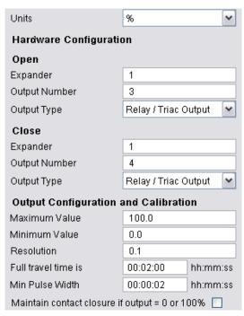
In this example, the controller turns off the signal to the appropriate output after the actuator reaches its fully open or fully closed position because **Maintain contact closure if current position = 0% or 100%** is not checked.
