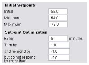
If the microblock outputs  $57^{\circ}$  and 5 minutes later the **req** input sees 4 requests, the new setpoint is  $56^{\circ}$  = (57 + 1 + (-2)).
