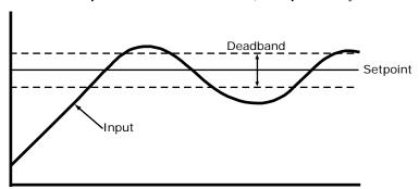
**NOTE** Once the **Input** falls outside the **Deadband**, it must reach or exceed the **Setpoint** value before the **Output** is paused again.
