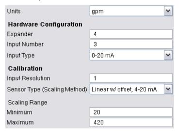
**NOTE** An input resolution of 1 causes the microblock to output gpm in whole numbers.
