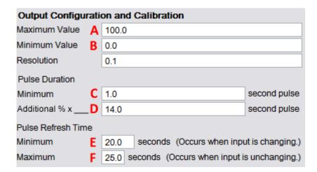
Pulse Duration varies linearly between 1 second and 1+14=15 seconds as the microblock input value varies from 0% (**Minimum Value**) to 100% (**Maximum Value**).
