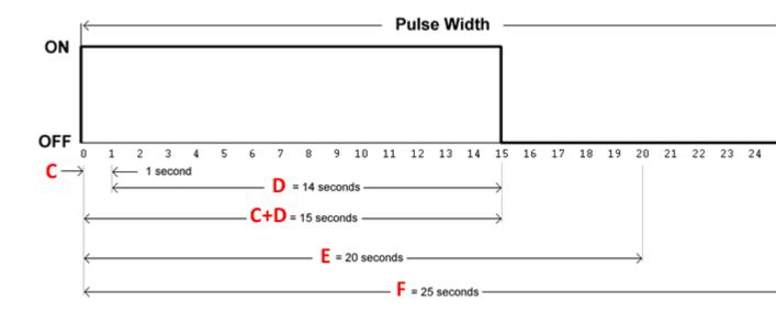
If the microblock input value changes by more than the **Resolution**, the microblock completes the current pulse, then recalculates and changes the pulse duration after the **Minimum Pulse Refresh Time**.
