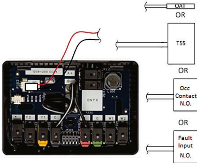
Match wire colors when connecting thermostat to sensor.
