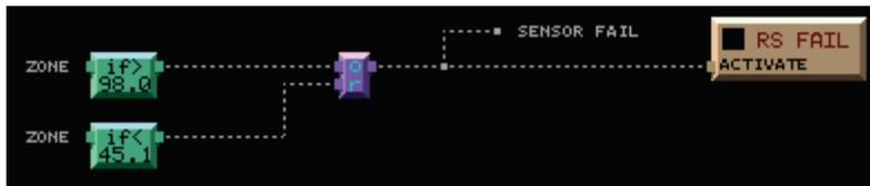
If the SPT sensor is used in a critical application, this logic will detect if the sensor is disconnected ( $<45.1^{\circ}\text{F}$ ) or is shorted ( $>98^{\circ}\text{F}$ ). The **Sensor Fail** label can be used to cause the control program to go into an appropriate failure mode if the sensor fails.
