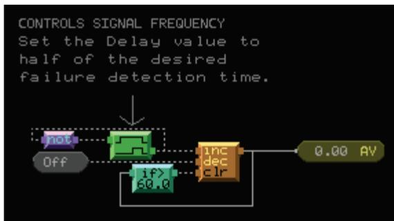
The logic in the network input's control program that receives the changing value. The SIGNAL analog network input's **Address** field contains the address of the BACnet Analog Value microblock sending the changing signal, and the network input's **Refresh Time** is 31 seconds.
