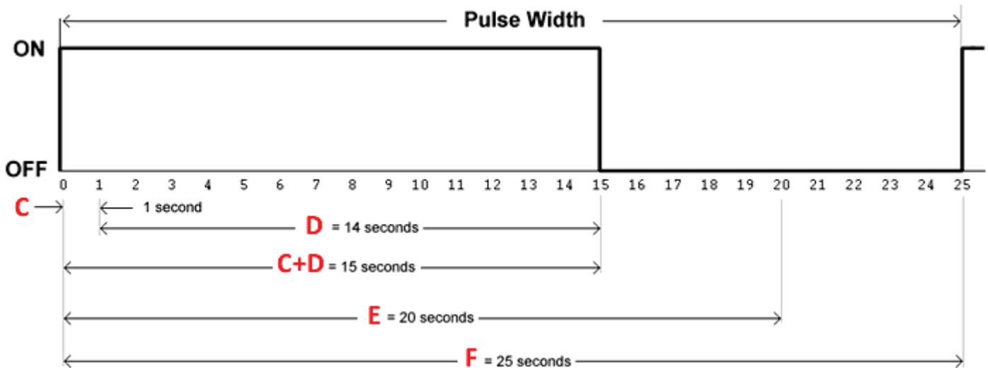
If the microblock input value changes by more than the **Resolution**, the microblock completes the current pulse, then recalculates and changes the pulse duration after the **Minimum Pulse Refresh Time**.
