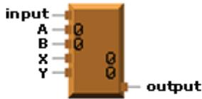
$$\text{output} = X + (\text{input} - A) * \frac{(Y - X)}{(B - A)}$$
