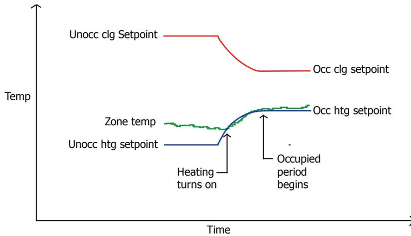
**Heating capacity calculation during optimal start**
