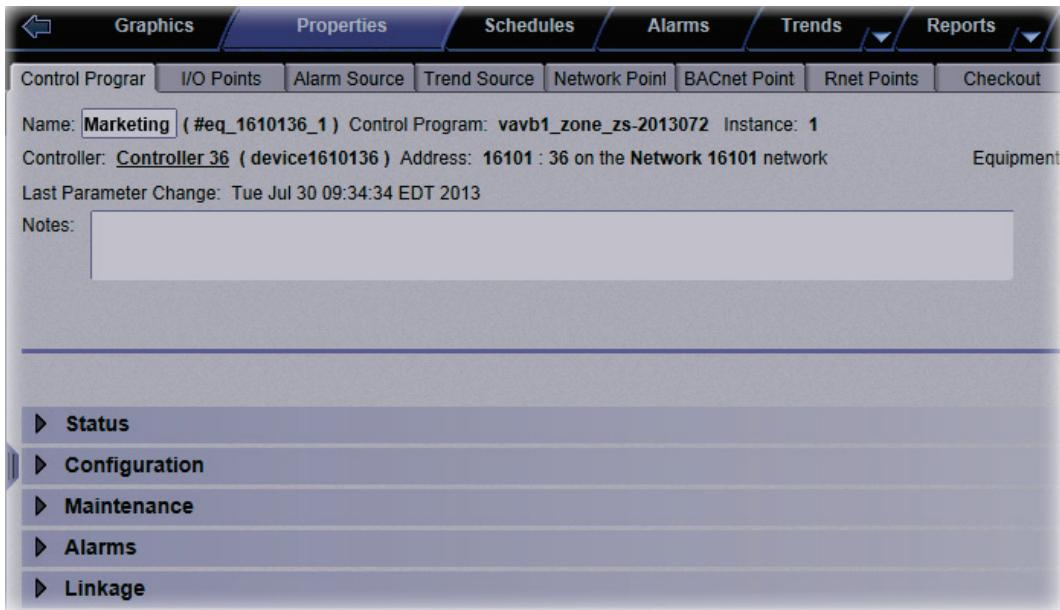
In the control program, you can change the way text appears on the **Properties** page by using a **Text** microblock or by editing a microblock's **Property Page Text** field in the **Property Editor**.
