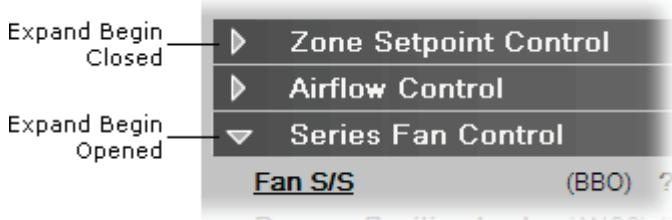
You must also insert a **Text** microblock with the **Text Type** set as **Expand End** at the end of the section you wish to group together.
