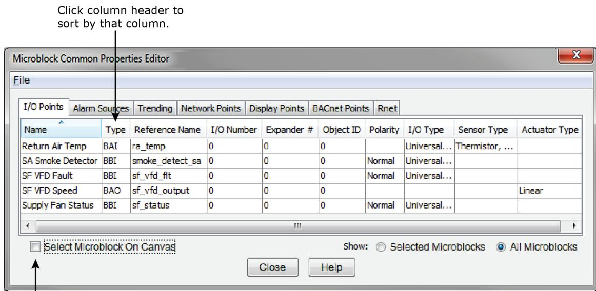
Select this checkbox and then select a point in the list to locate that microblock in the control program.
