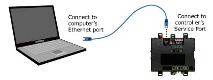
If your computer uses a static IP address, set the address to 169.254.1.x, where x is 2 or greater. If it uses a DHCP address, leave the address as it is.
