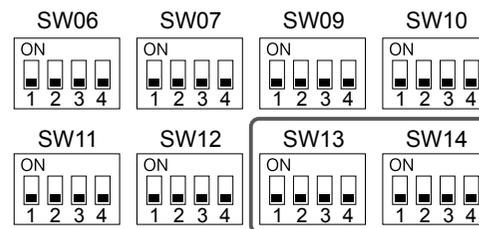
Switch settings for a line (system) address on the interface P.C. board for the outdoor unit
