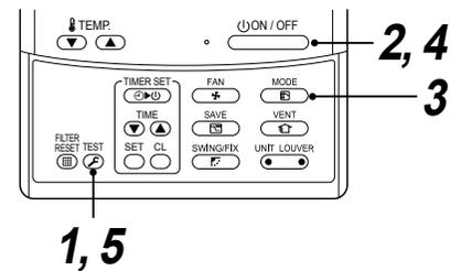
1 Push and hold the **TEST** button for more than 4 seconds. **TEST** appears on the LCD and the unit enters the **TEST** mode.
