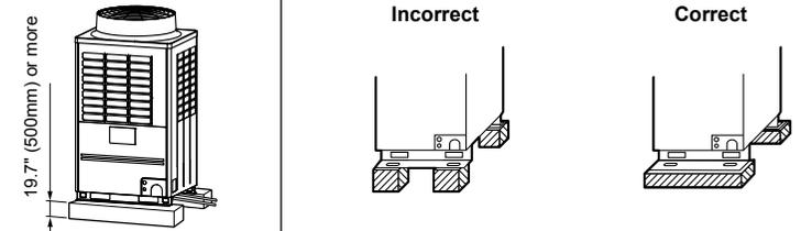
4. If vibration-proof rubbers (including vibration-proof blocks) are used, fit them under the whole clamping legs.
