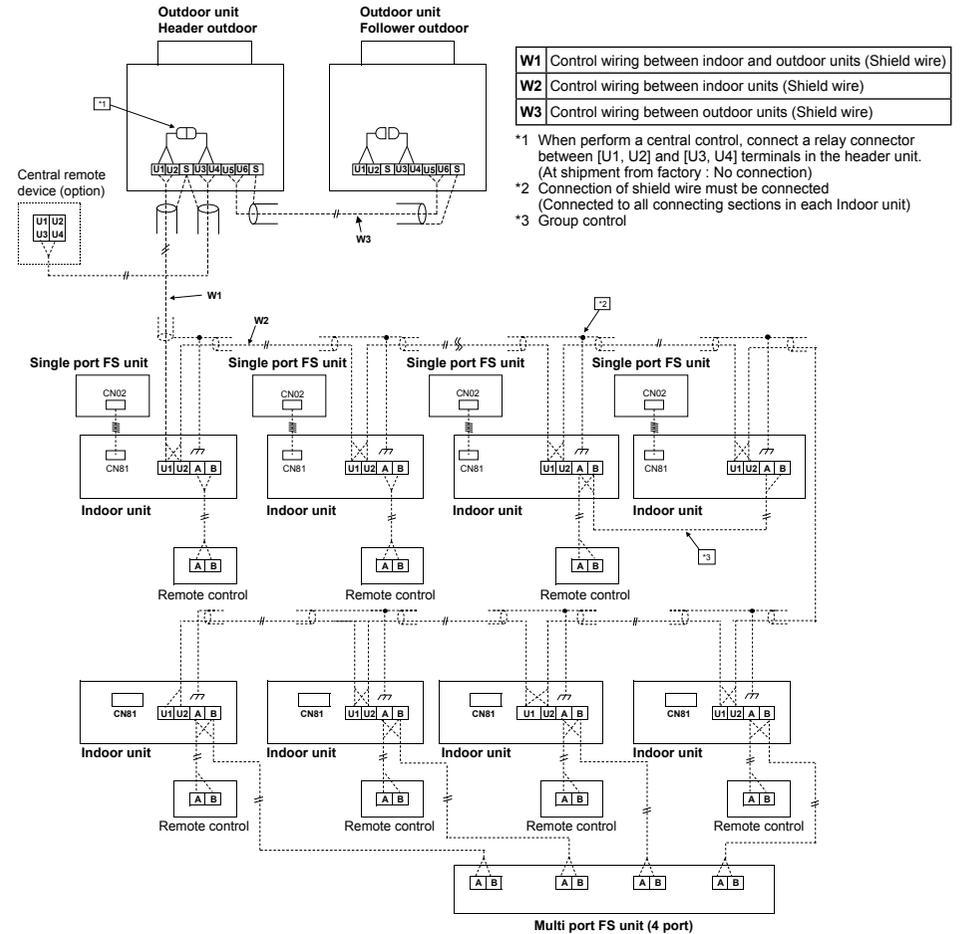
1. All system interconnecting and central control wiring should be 2 conductor shielded cable.
