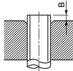
**Extruding margin of copper pipe with flare tools: A (Unit: in (mm))**
