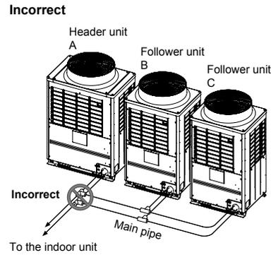
**When drawing pipes downward**
