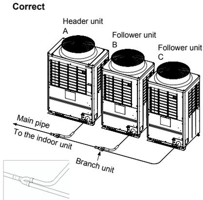
[Inverse connection of a gas-side branch unit]
