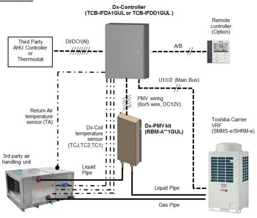
Refrigerant piping (Maximum piping length from Dx-PMV kit to 3<sup>rd</sup> party coil : 16ft)
