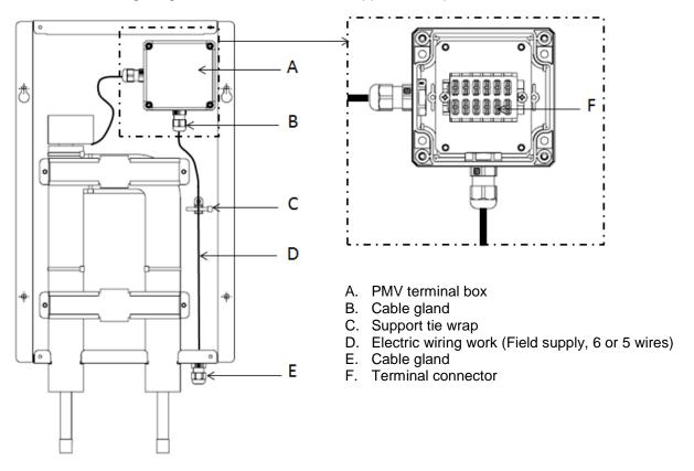
PMV (Pulse motor wiring)
