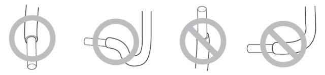
•Make good between temperature sensor and Dx-coil. Put the top of the thermistors on the Dx-Coil, this is the most sensitive point of the sensor.
