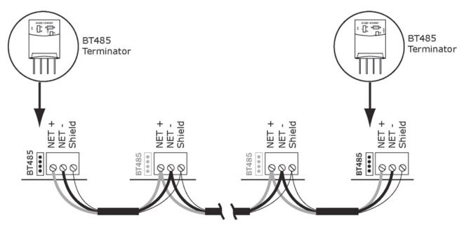
Fig. 38 — Network Wiring
