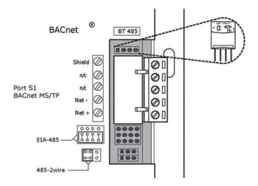
Fig. 39 — BT485 Terminator Installation
