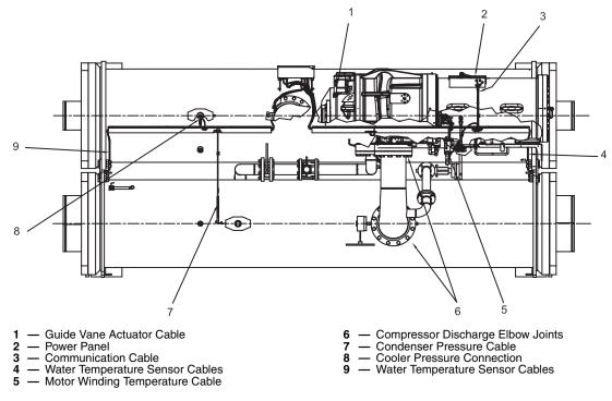
Fig. 8 — 19XR Chiller Top View
