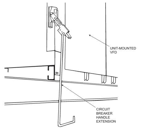
Fig. 24 — Circuit Breaker Handle Extension Installed
