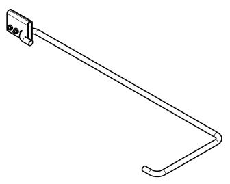
Fig. 23 — Circuit Breaker Handle Extension
