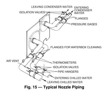
option; however, water piping should not cross in front of the waterbox or access will be blocked.
