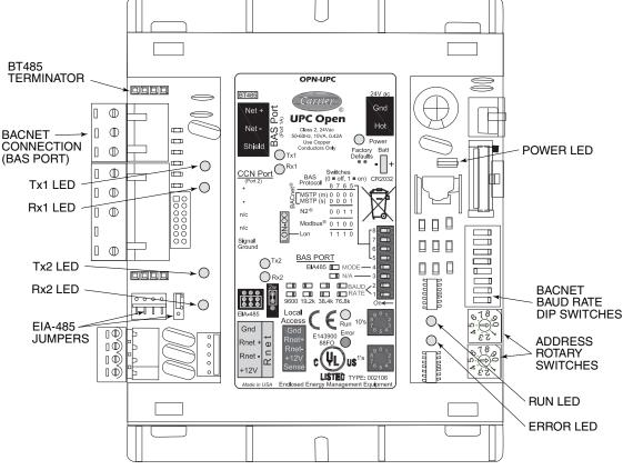
Fig. 37 — UPC Open Controller
