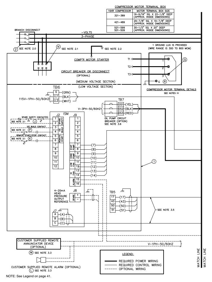
Fig. 31 — 19XR Typical Field Wiring with Free-Standing Starter (Medium Voltage)
