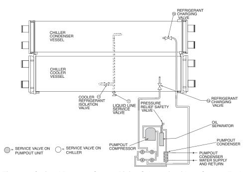
Fig. 20 — Optional Pumpout System Piping Schematic without Storage Tank
