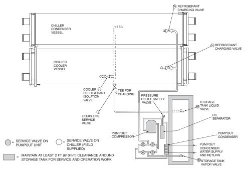
Fig. 19 — Optional Pumpout System Piping Schematic with Storage Tank
