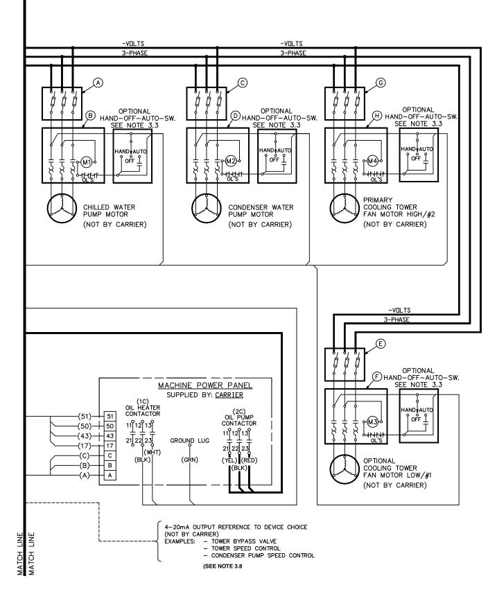
Fig. 32 — 19XR Typical Field Wiring with Free-Standing Low Voltage VFD (cont)
