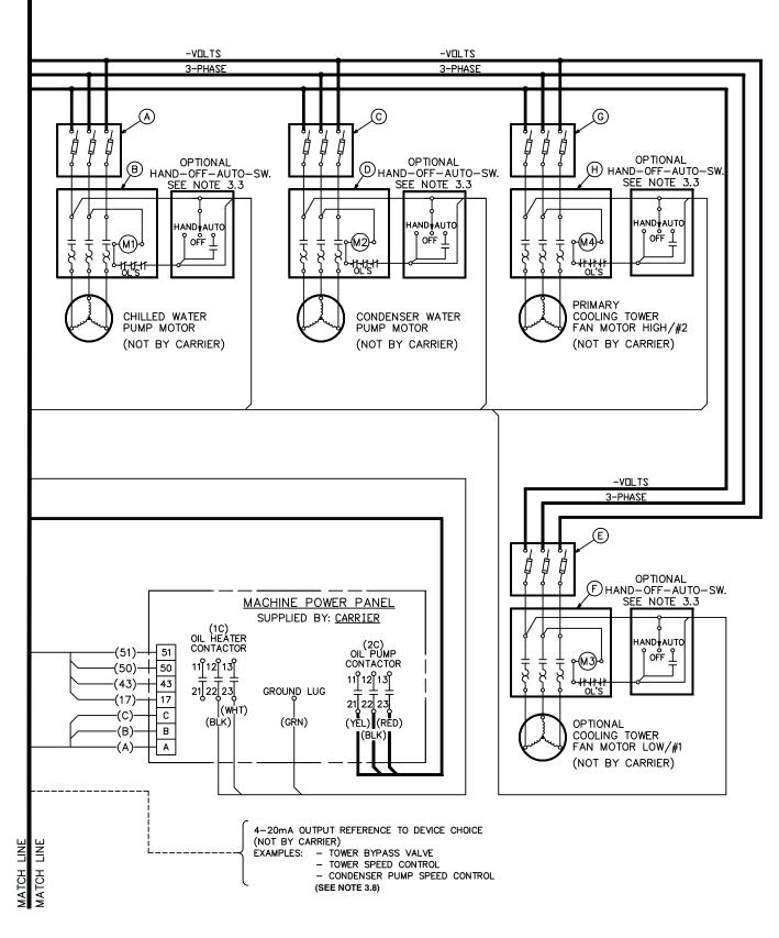
Fig. 31 — 19XR Typical Field Wiring with Free-Standing Starter (Medium Voltage) (cont)
