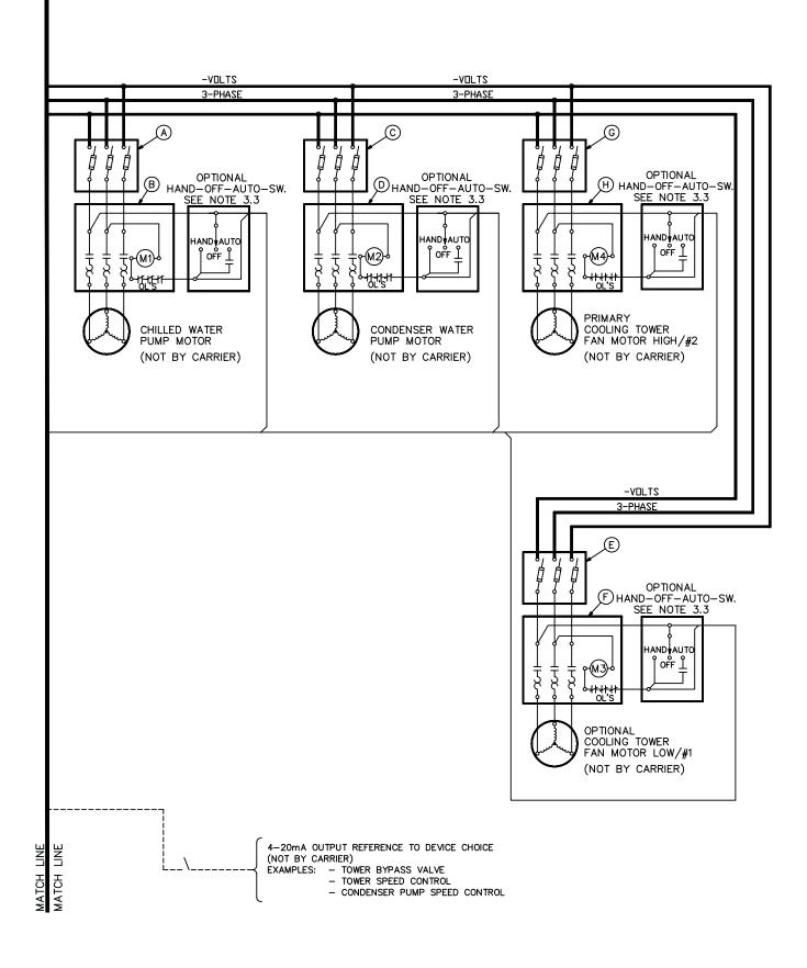
Fig. 28 — 19XR Typical Field Wiring with Unit-Mounted Starter (Benshaw Starter Shown) (cont)
