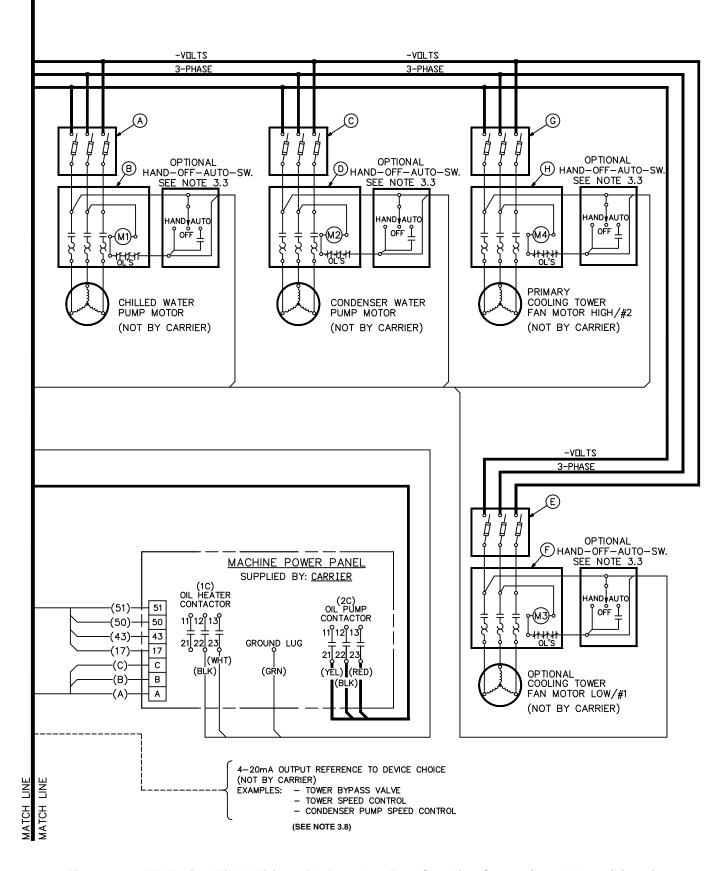
Fig. 30 — 19XR Typical Field Wiring with Benshaw Free-Standing Starter (Low Voltage) (cont)
