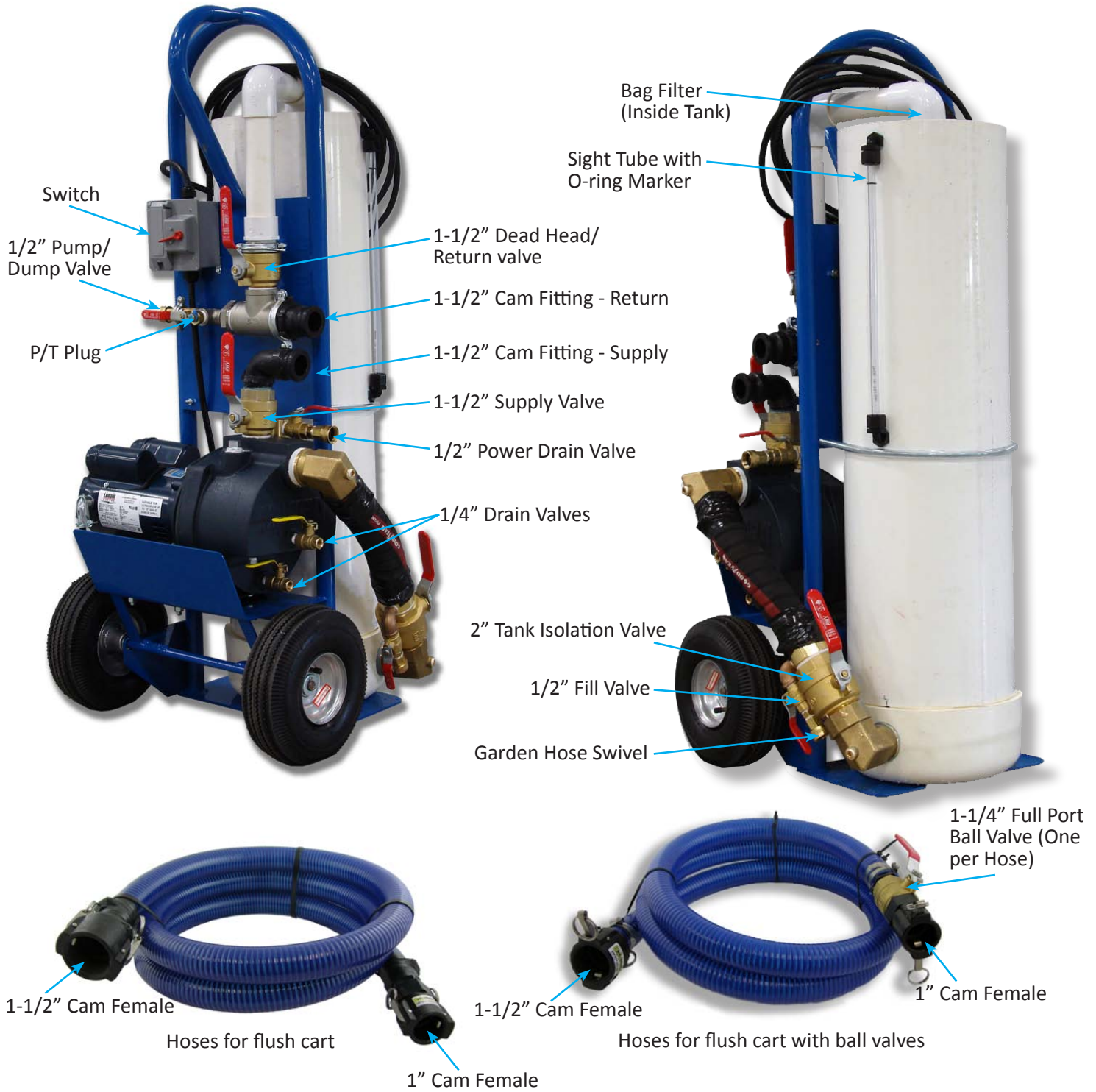
Figure 11: Flush cart diagram with descriptions
