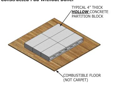
Figure 1 - Boiler Placement On Constructed Pad
