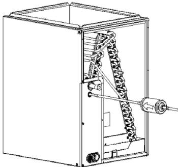
Fig. 3 - Liquid Line Filter Drier
