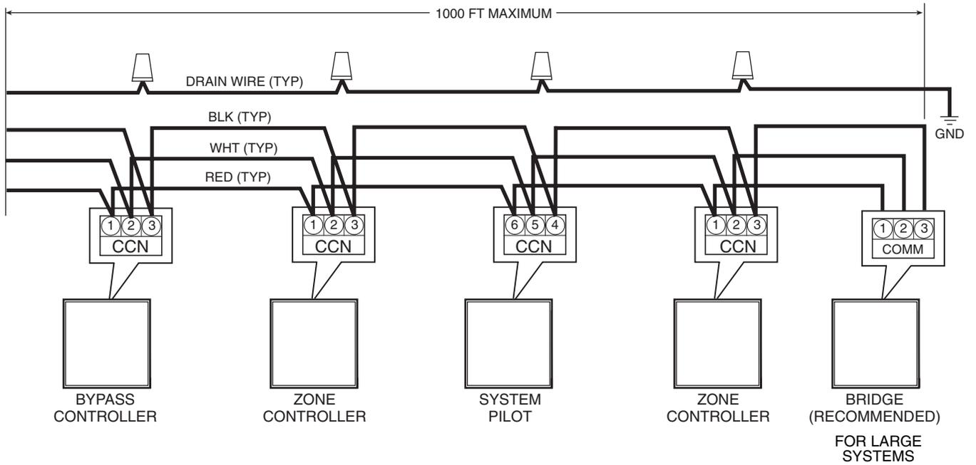
→Fig. 3 — Carrier Communicating Network Communication Bus Wiring
