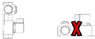
Figure 5. Flow center must be installed so that the pump's shaft is horizontal.
