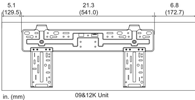
Fig. 10 – 9k & 12k Mounting Plate Spacing
