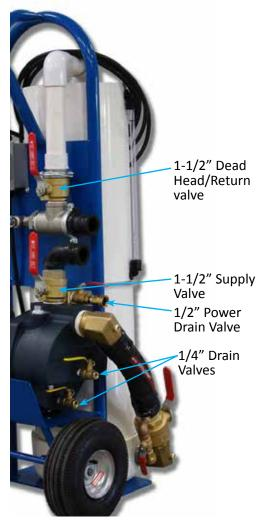
Figure 12: Flush Cart Valves in flushing steps
