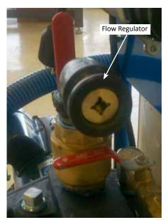
Figure 3: Flow regulator installed in 1-1/2" cam supply
