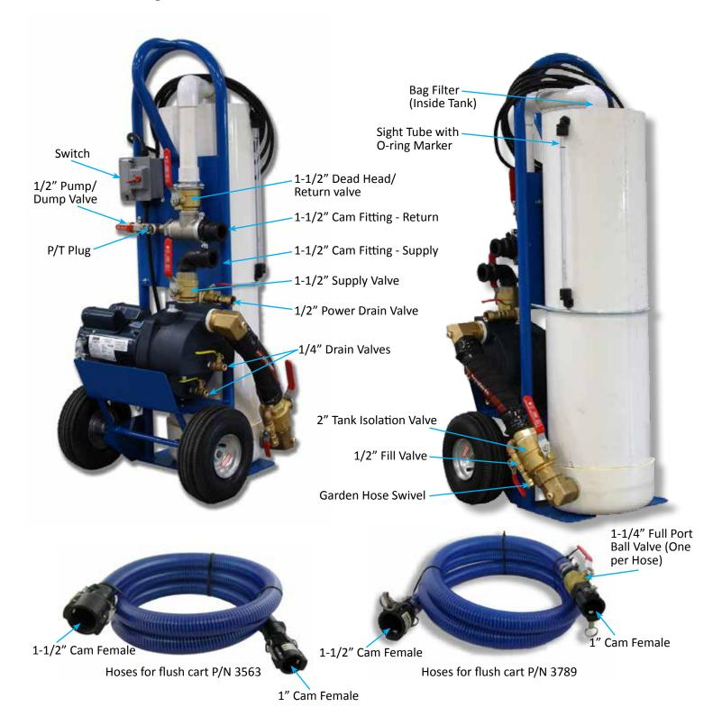
Figure 2: Flush cart diagram with descriptions
