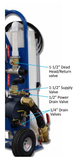
Figure 21: Flush Cart Valves in emptying the tank
