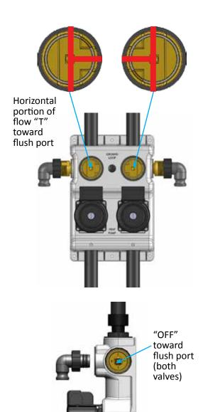
Figure 11: FPT flow center (top) and Flo-Link Double O-ring flow center (below) valve positions in operating position
