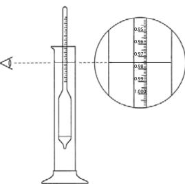
Figure 16: Typical hydrometer (above); reading a hydrometer (below). In the example, this hydrometer would be read as 0.975, approximately 24% ethanol by volume. NOTE: There are two types of hydrometers, one for fluids lighter than water (ethanol and methanol); and one for fluids heavier than water (propylene glycol).
