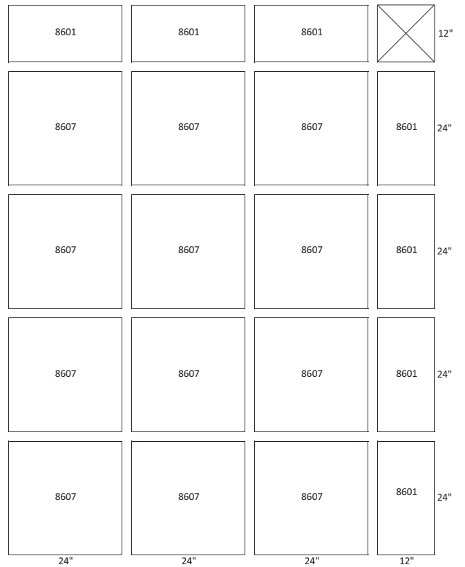
UNIT SIZE: 58T (12) 24" X 24" FILTERS (7) 12" X 24" FILTERS
