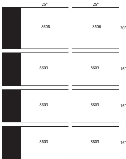
UNIT SIZE: 22T (2) 20" X 25" FILTERS (6) 16" X 25" FILTERS
