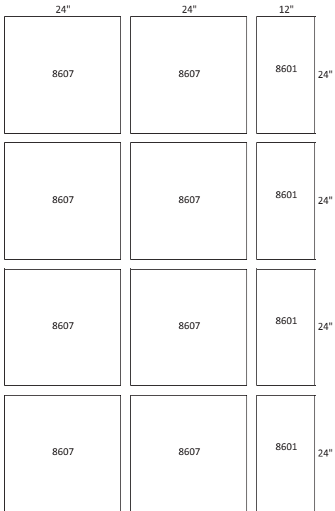
UNIT SIZE: 37T (8) 24" X 24" FILTERS (4) 12" X 24" FILTERS
