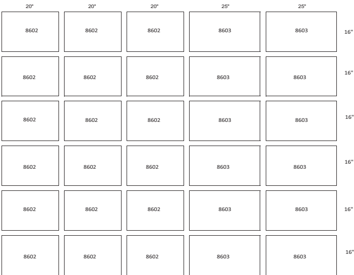
UNIT SIZE: 50W (18) 16" X 20" FILTER (12) 16" X 25" FILTER
