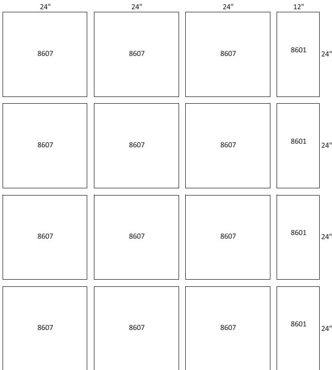
UNIT SIZE 51T (12) 24" X 24" FILTERS (4) 12" X 24" FILTERS
