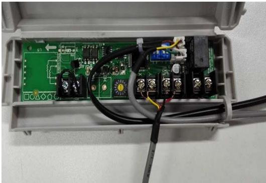
**Fig. 26 — Connect the cable to the board**
