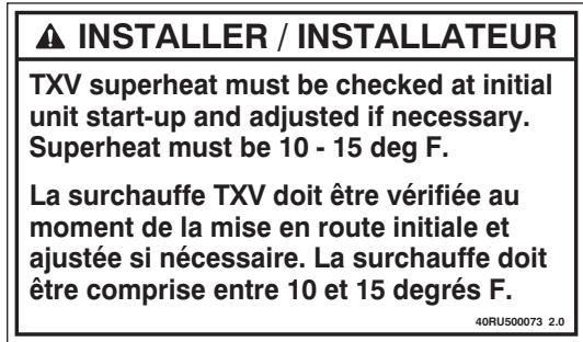
Fig. 21 - Label, TXV Adjustment
