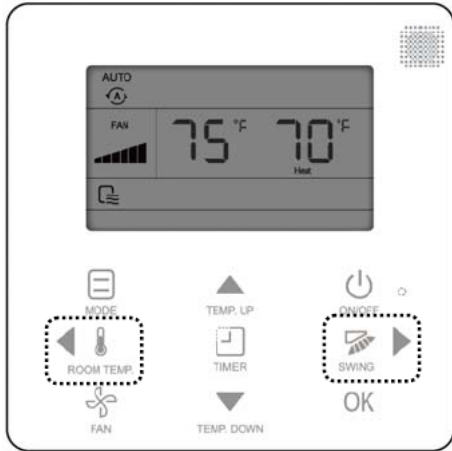
Fig. 13 — Switching Between Cooling and Heating
