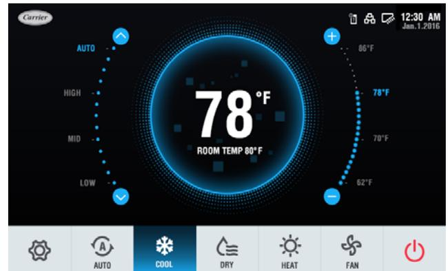
**Fig. 28 —Indoor Temperature Display on Homepage**
