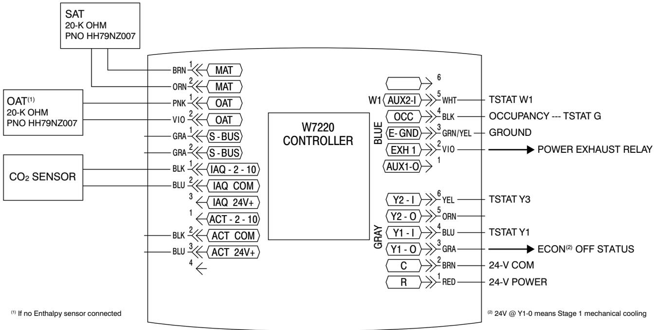
Fig. 58 - W7220 Sensor and Control I/O Connections
