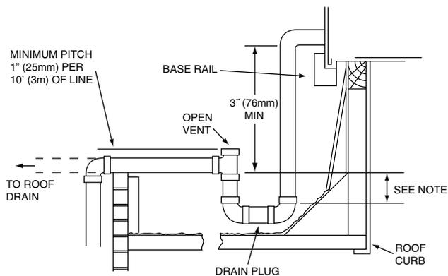
NOTE: Trap should be deep enough to offset maximum unit static difference. A 4" (102mm) trap is recommended.
