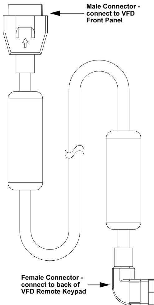
**Fig. 71 - VFD Remote Keypad Cable**
