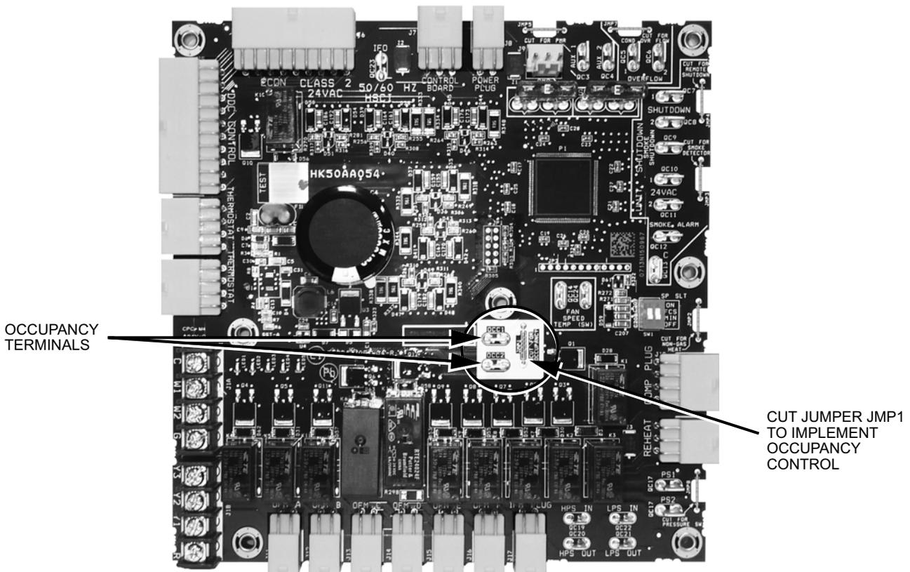
Fig. 63 - Integrated Staging Control (ISC) Board - Occupancy Terminals and Jumper
