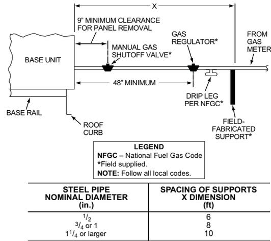
**Fig. 17 - Gas Piping Guide**
