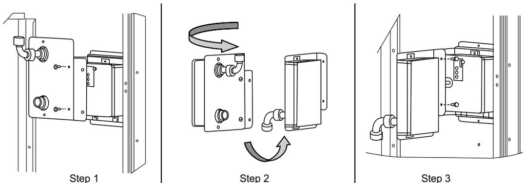
Fig. 74 - Completing Installation of Return Air Smoke Sensor
