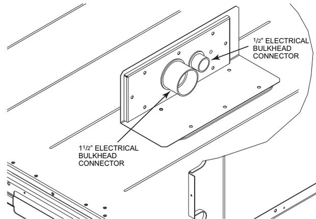
**Fig. 47 - Thru-the-Base Option, Shipping Position**
