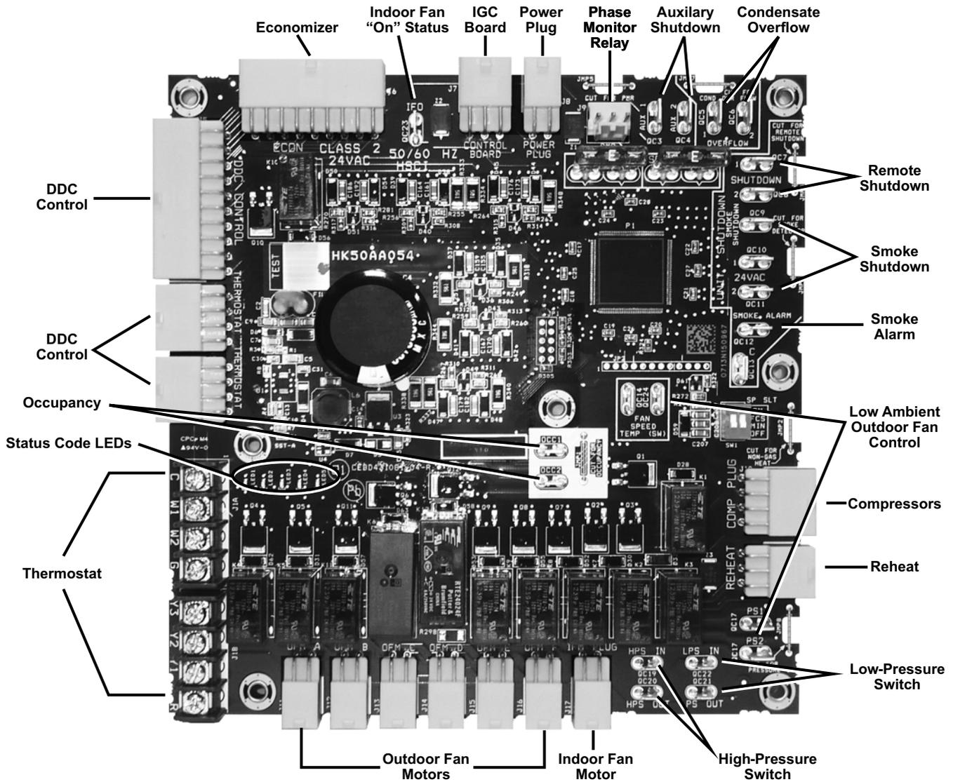
Fig. 53 - Integrated Staging Control (ISC) Board
