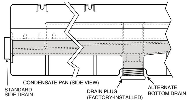
Fig. 25 - Condensate Drain Pan (Side View)
