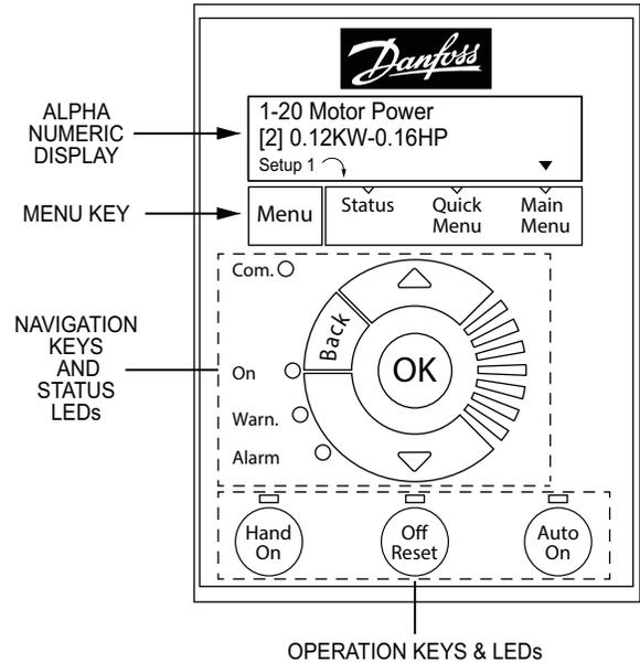
**Fig. 68 - VFD Keypad**
