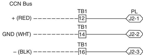
**Fig. 92 — PremierLink CCN Bus Connections (Sizes 08-14 Shown)**
