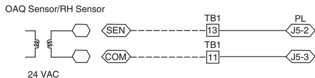
**Fig. 85 — Outdoor CO<sub>2</sub> Sensor Connections (Sizes 08-14 Shown)**
