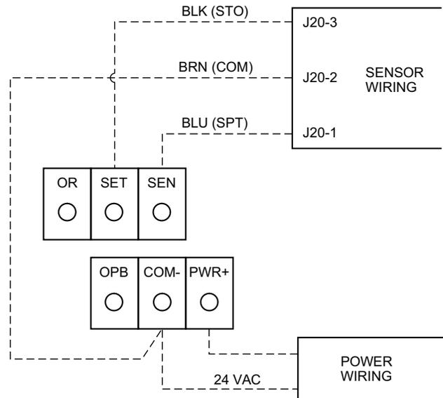
NOTE: Must use a separate isolated transformer.
