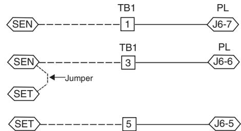
**Fig. 80 — PremierLink T-56 Sensor (Sizes 08-14 Shown)**
