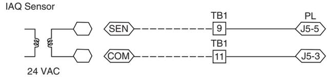
**Fig. 83 — Indoor CO<sub>2</sub> Sensor (33ZCSENC02) Connections (Sizes 08-14 Shown)**
