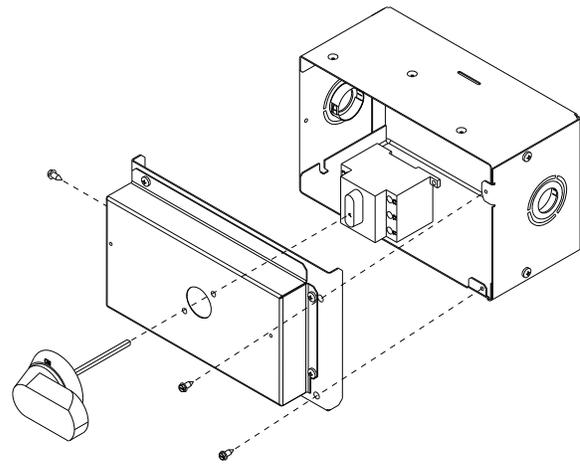
**Fig. 46 — Handle and Shaft Assembly for NFD (Sizes 08-14)**
