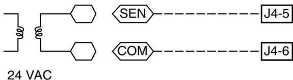
**Fig. 103 — RTU Open / Outdoor CO<sub>2</sub> Sensor (33ZCSENCO2) Connections**
