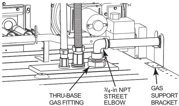
**Fig. 30 — Gas Line Piping (Size 16)**
