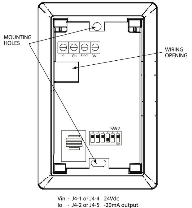
**Fig. 104 — Space Relative Humidity Sensor Typical Wiring**
