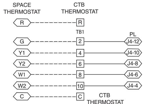
**Fig. 81 — Space Thermostat Connections (Sizes 08-14 Shown)**
