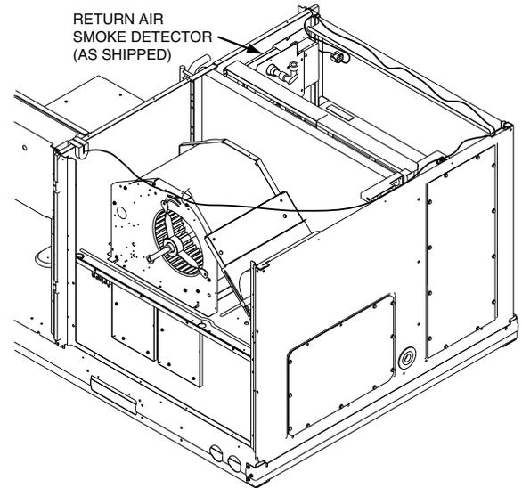
**Fig. 112 — Return Air Smoke Detector; Shipping Position**
