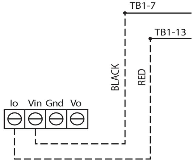
**Fig. 87 — Space Relative Humidity Sensor Connection (Sizes 08-14 Shown)**
