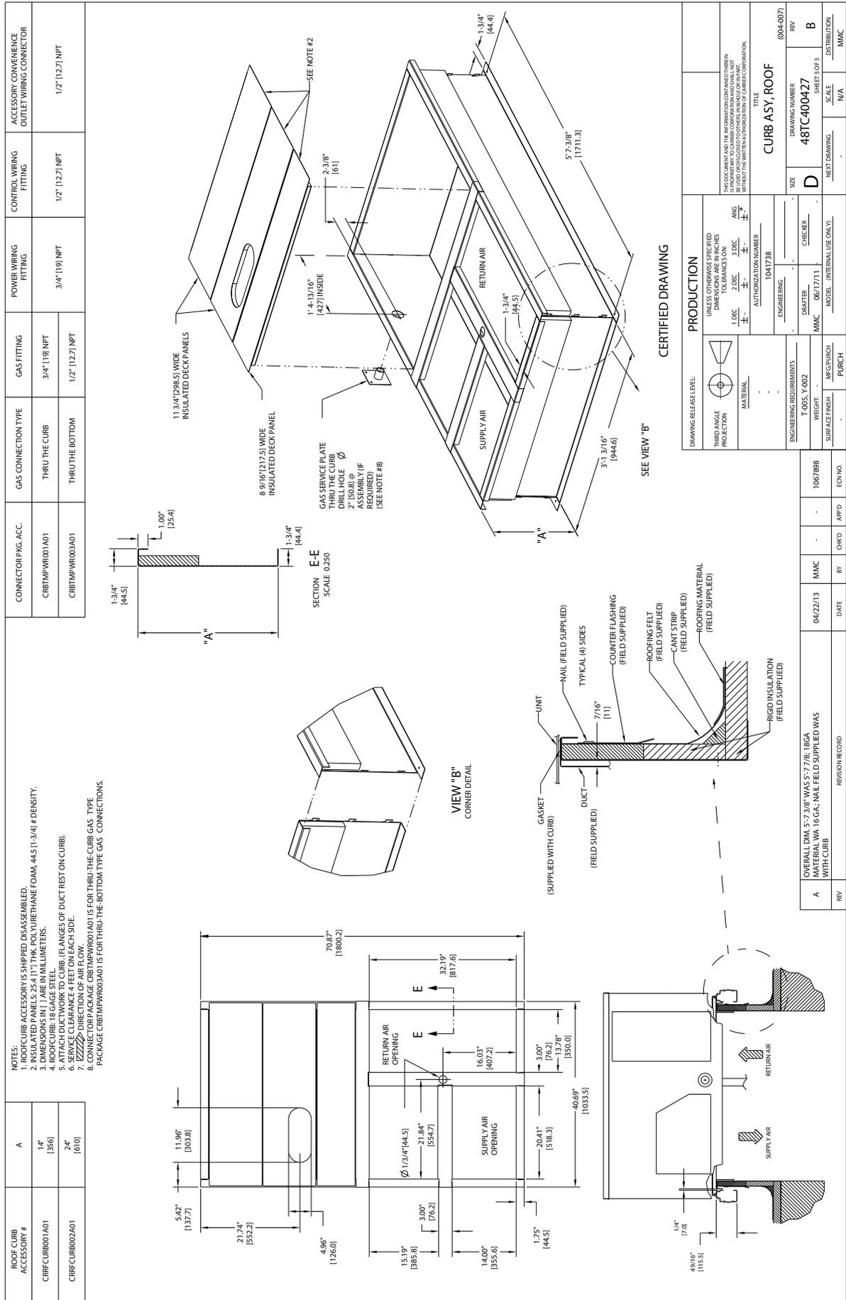
Fig. 8 — 48TC\*\*08-14 — Roof Curb Details
