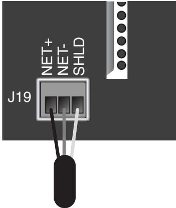
Fig. 108 — Network Wiring
