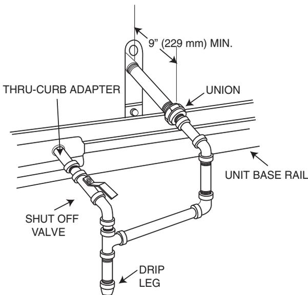
**Fig. 31 — Gas Piping with Thru-Curb Accessory**
