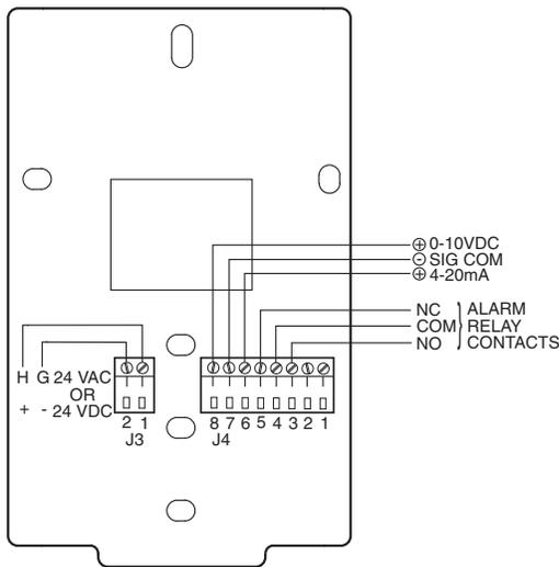
**Fig. 82 — Indoor/Outdoor Air Quality (CO<sub>2</sub>) Sensor (33ZCSENC02) — Typical Wiring Diagram**
