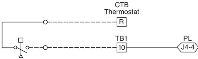
**Fig. 88 — PremierLink Filter Switch Connection (Sizes 08-14 Shown)**
