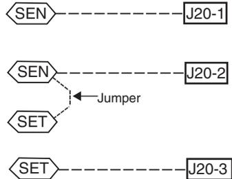
**Fig. 100 — RTU Open T-56 Sensor Connections**
