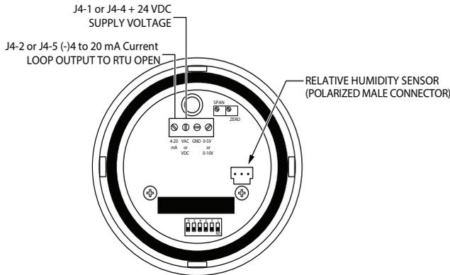
**Fig. 105 — Duct Relative Humidity Sensor Typical Wiring**
