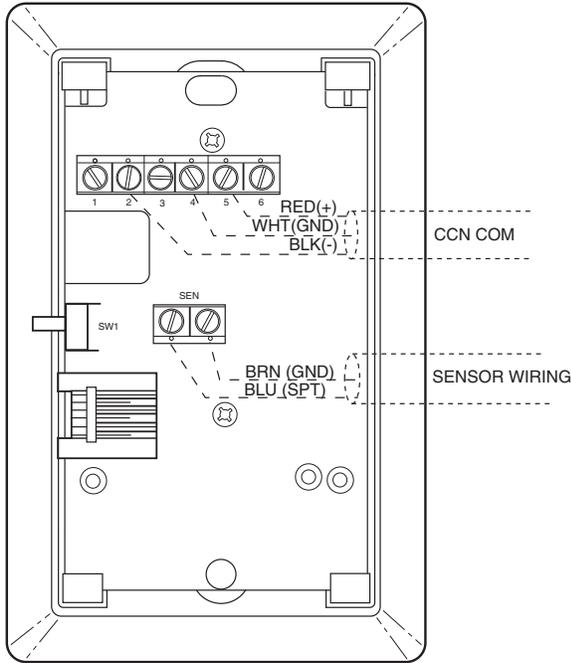
**Fig. 77 — T-55 Space Temperature Sensor Wiring**
