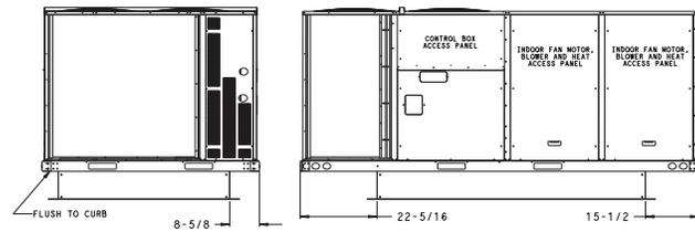
**Fig. 11 — Retrofit Installation Dimensions (Size 16 Shown)**
