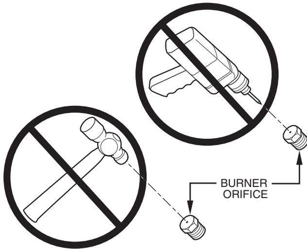
**Fig. 34 — Orifice Hole**
