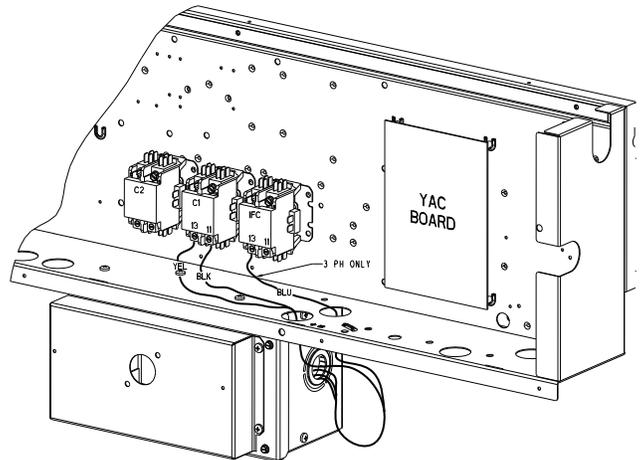
**Fig. 44 — Location of Non-Fused Disconnect Enclosure (Sizes 08-14)**
