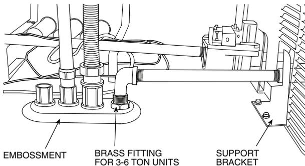
**Fig. 27 — Gas Line Piping (Sizes 08-14)**
