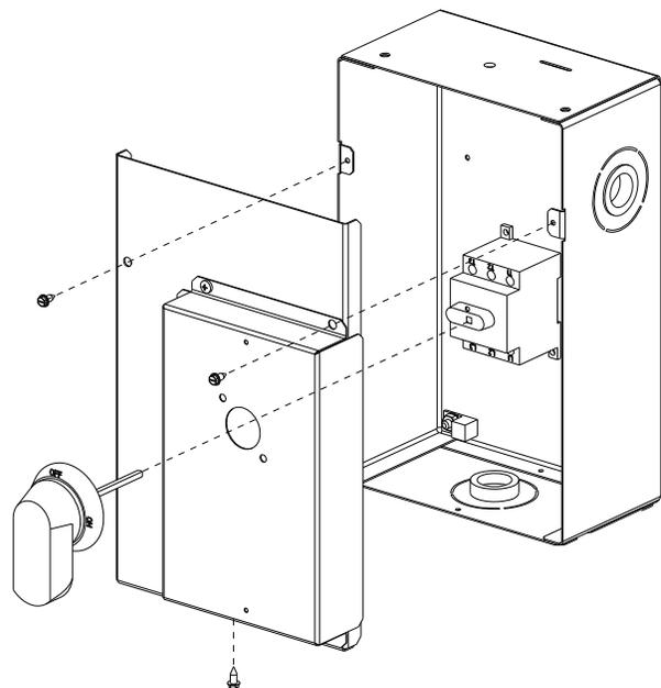
**Fig. 47 — Handle and Shaft Assembly for NFD (Size 16)**
