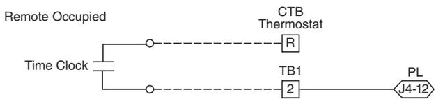
**Fig. 90 — PremierLink Wiring Remote Occupied (Sizes 08-14 Shown)**
