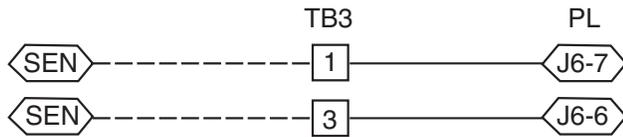
**Fig. 78 — PremierLink T-55 Sensor (Sizes 16 Shown)**
