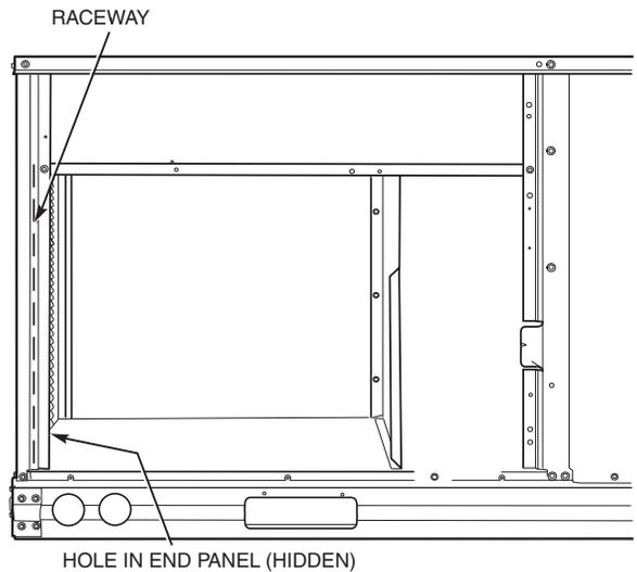
**Fig. 54 — Field Control Wiring Raceway (08-14 Only)**
