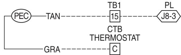
**Fig. 91 — PremierLink Power Exhaust Output Connection (Sizes 08-14 Shown)**
