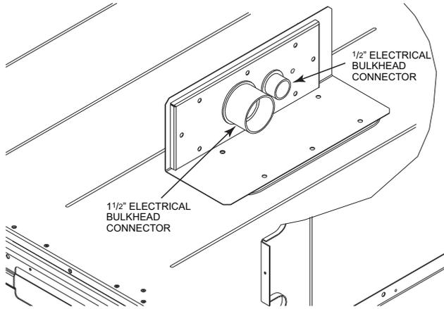
**Fig. 55 — Thru-the-Base Option, Shipping Position (Size 16)**
