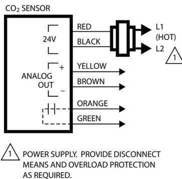
**Fig. 66 — CO<sub>2</sub> Sensor Wiring**
