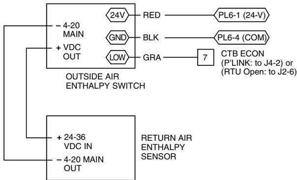
**Fig. 111 — Outside and Return Air Enthalpy Sensor Wiring**
