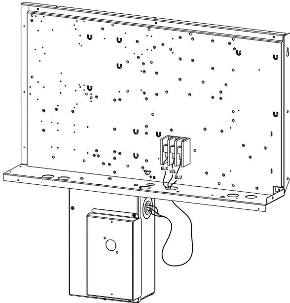
**Fig. 45 — Location of Non-Fused Disconnect Enclosure (Sizes 16)**
