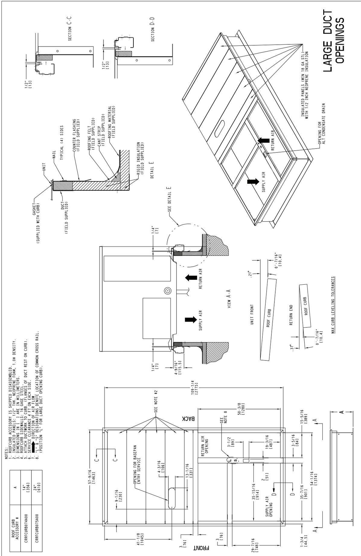
Fig. 9 — 48TC\*\*16 — Roof Curb Details
