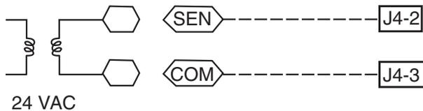
**Fig. 102 — RTU Open/Indoor CO<sub>2</sub> Sensor (33ZCSENCO2) Connections**
