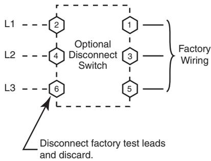
**Fig. 37 — Power Wiring Connections (Sizes 08-14)**
