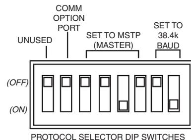
**Fig. 106 — RTU Open SW3 DIP Switch Settings**
