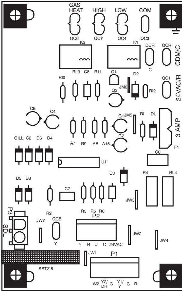
Fig. 21 - Interface Fan Board (IFB) 460 VAC Models
