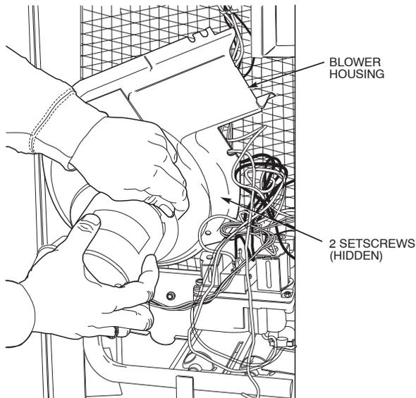
Fig. 24 - Removal of Motor and Blower Wheel
