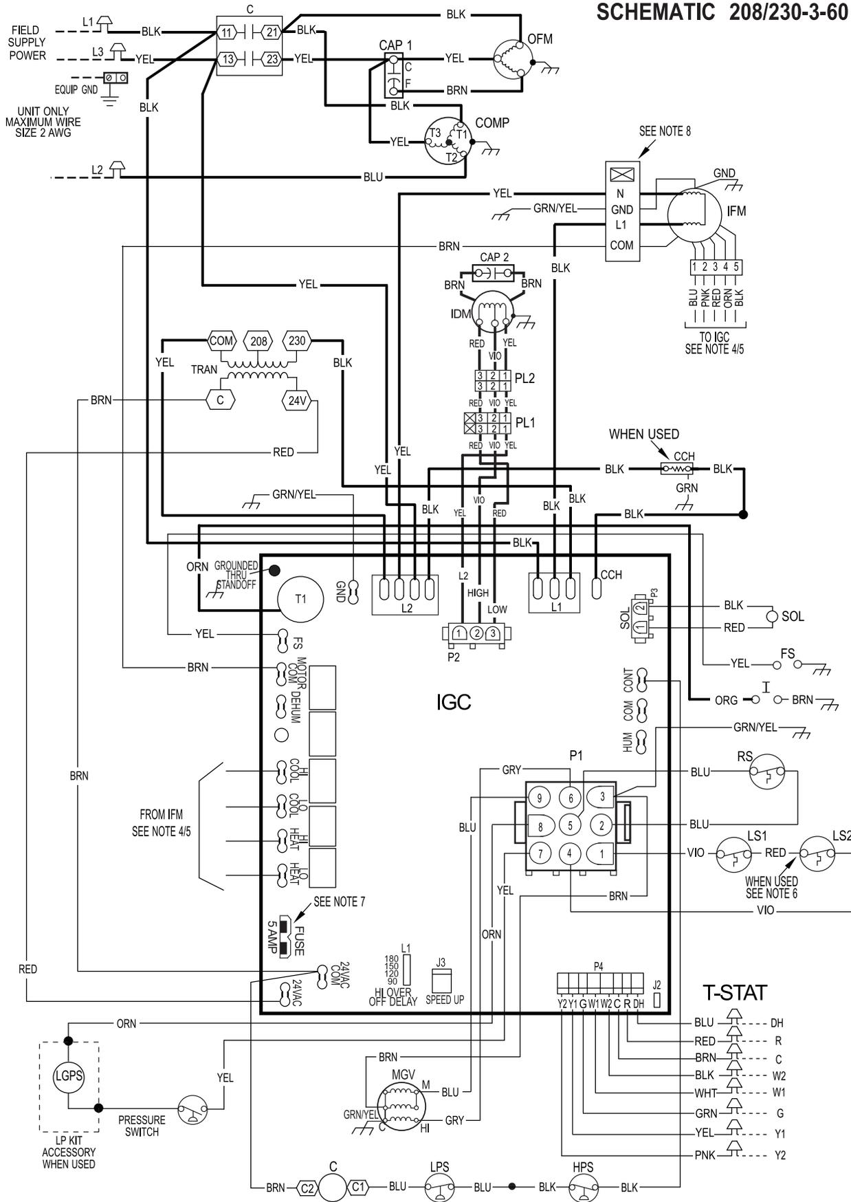
**Fig. 17 - 208/230-3-60 Connection Wiring Diagram Gas Inputs 40, 60, 90 KBtu/hr**
