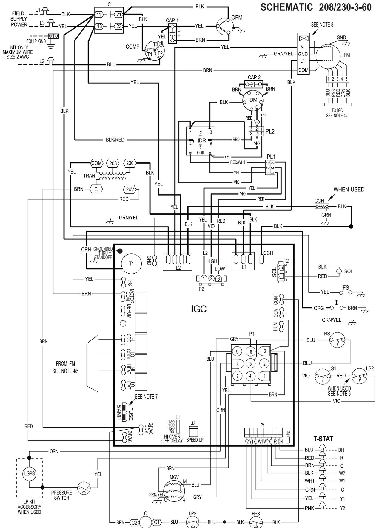
**Fig. 18 - 208/230-3-60 Connection Wiring Diagram Gas Inputs 115, 130**
