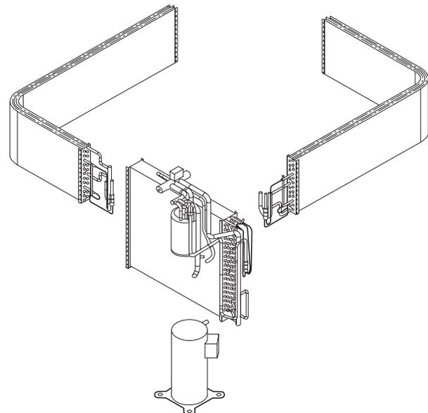
Fig. 26 - Refrigerant Circuit
