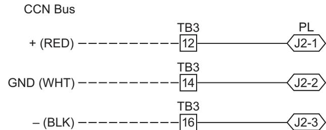
**Fig. 65 — PremierLink Controller CCN Bus Connections**
