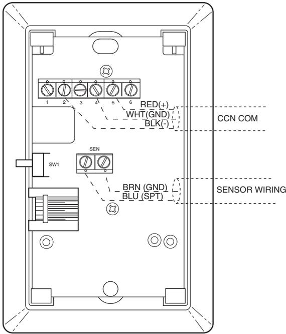
**Fig. 50 — T-55 Space Temperature Sensor Wiring**
