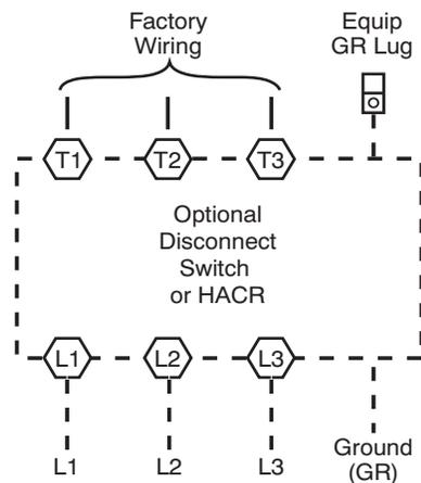
**Fig. 23 — Power Wiring Connections**
