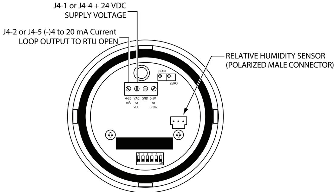
**Fig. 75 — Duct Relative Humidity Sensor Typical Wiring**
