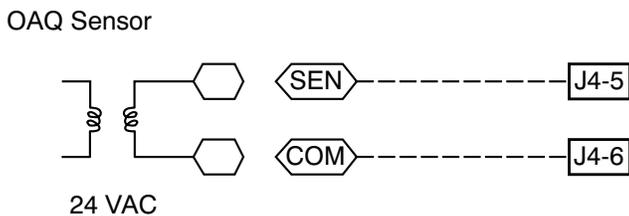
**Fig. 73 — RTU Open Controller/Outdoor CO<sub>2</sub> Sensor (33ZCSENC02) Connections**
