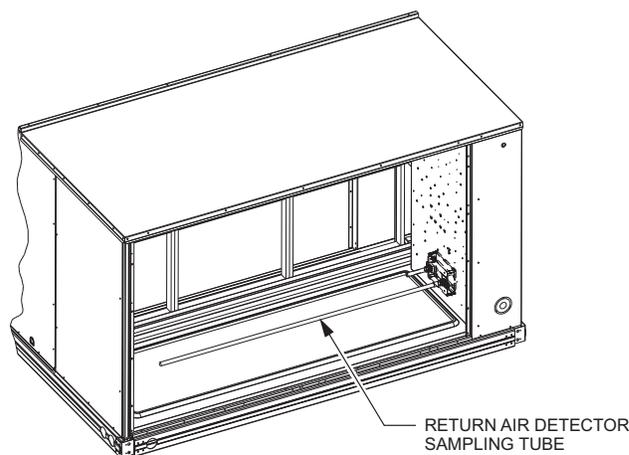
**Fig. 84 — Return Air Sampling Tube Location in Unit with Economizer**
