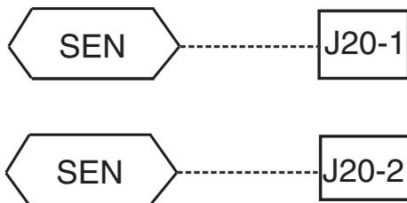
**Fig. 69 — RTU Open Controller T-55 Sensor Connections**
