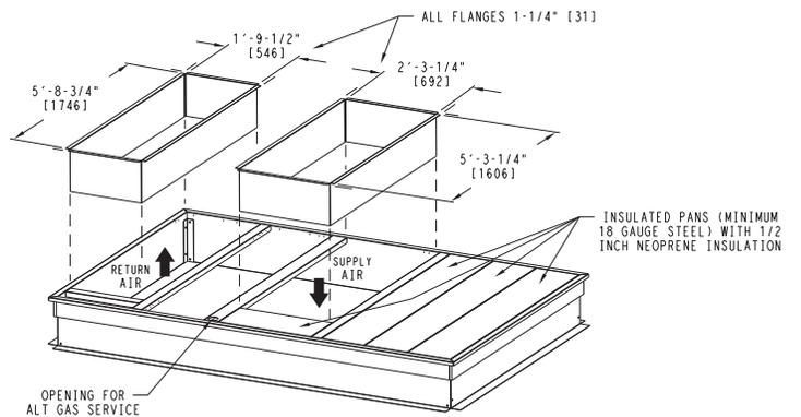
Fig. 8 — Roof Curb Details — 17 Size Unit
