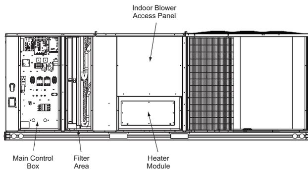
**Fig. 32 — Typical Component Location**
