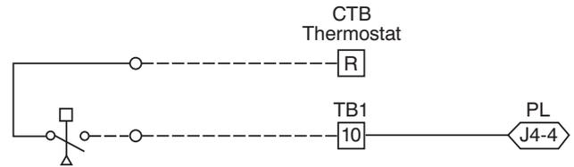
**Fig. 61 — PremierLink Controller Filter Switch Connection**
