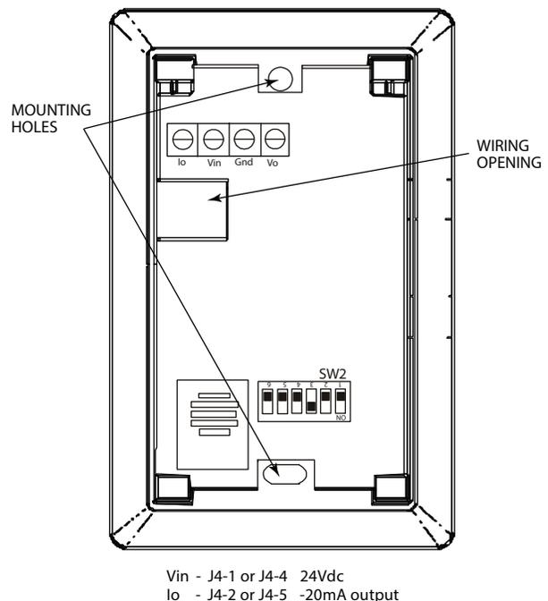
**Fig. 74 — Space Relative Humidity Sensor Typical Wiring**
