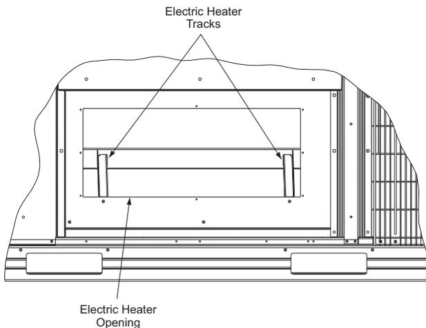
**Fig. 33 — Electric Heater Compartment (Cover Removed)**
