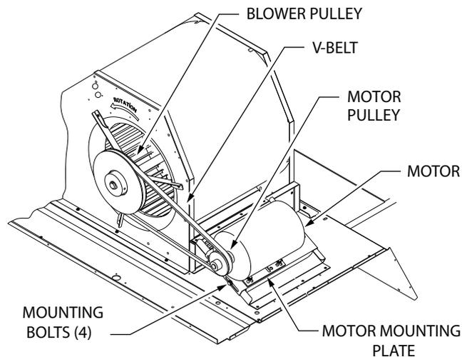
**Fig. 87 — Belt Drive Motor Mounting**
