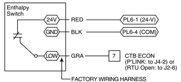
**Fig. 80 — Enthalpy Switch (33CSENTHSW) Connections**
