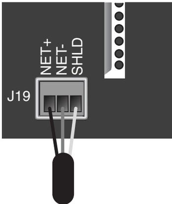
Fig. 78 — Network Wiring
