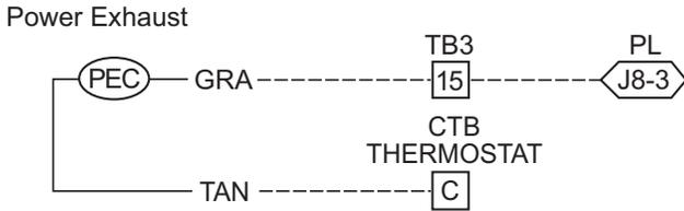
**Fig. 64 — PremierLink Controller Power Exhaust Output Connection**
