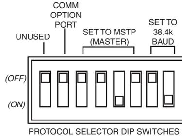
Fig. 76 — RTU Open Controller SW3 Dip Switch Settings
