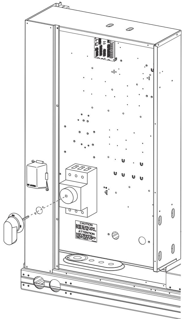
**Fig. 22 — Handle and Shaft Assembly for HACR**
