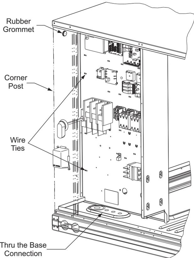
**Fig. 30 — Field Control Wiring Raceway**
