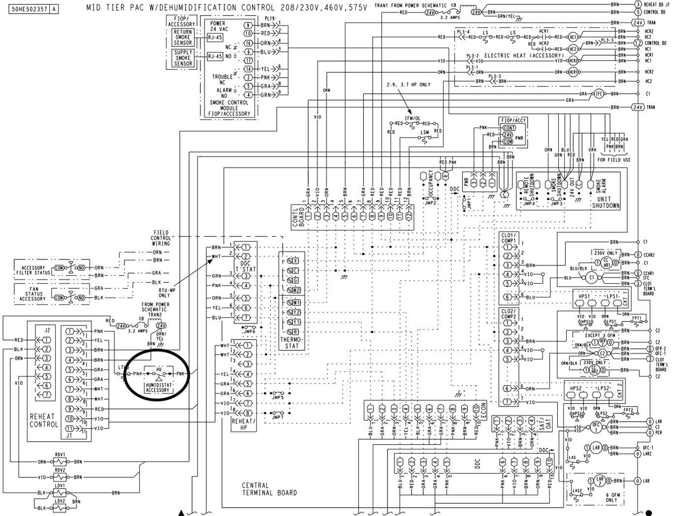
Fig. 37 — Typical Humidi-MiZer® Adaptive Dehumidification System Humidistat Wiring
