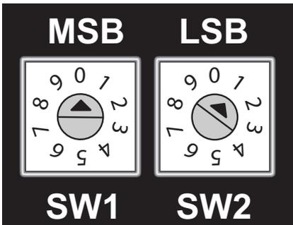
Fig. 77 — RTU Open Controller Address Switches
