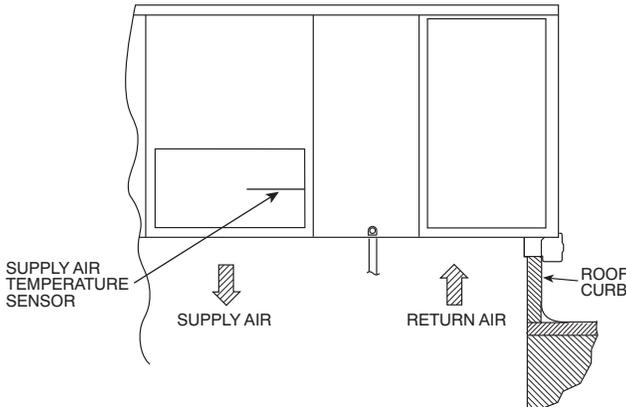
**Fig. 49 — Mounting Location for Supply Air Temperature (SAT) Sensor on 50HC Units**
