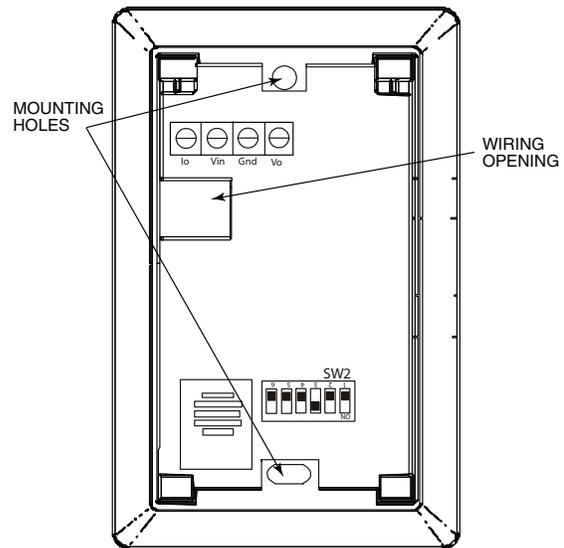
**Fig. 59 — Space Relative Humidity Sensor Installation**
