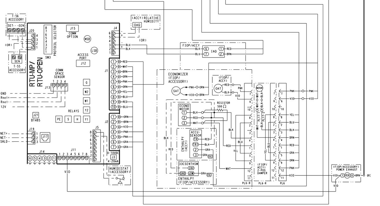
Fig. 67 — RTU Open System Control Wiring Diagram
