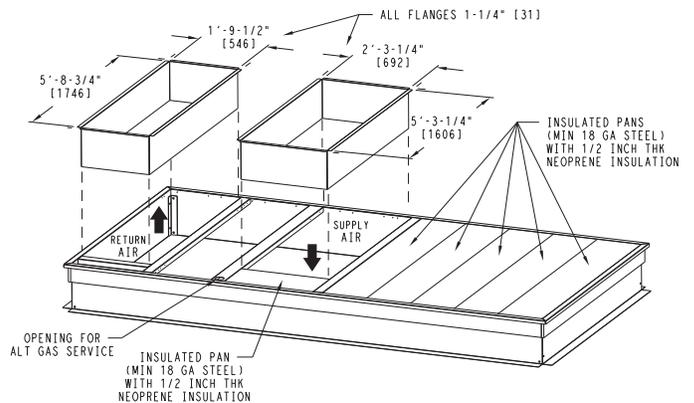
Fig. 10 — Roof Curb Details — 28 Size Unit
