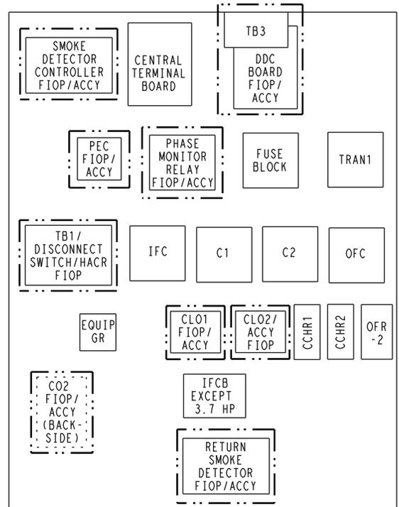
**Fig. 46 — 50HC Control Box Component Locations**
