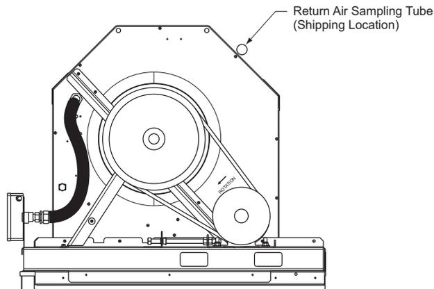
**Fig. 82 — Typical Supply Air Smoke Detector Sensor Location**
