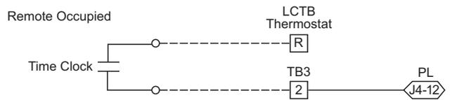
**Fig. 63 — PremierLink Controller Wiring Remote Occupied**
