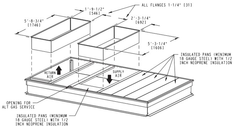
Fig. 9 — Roof Curb Details — 20 and 24 Size Units
