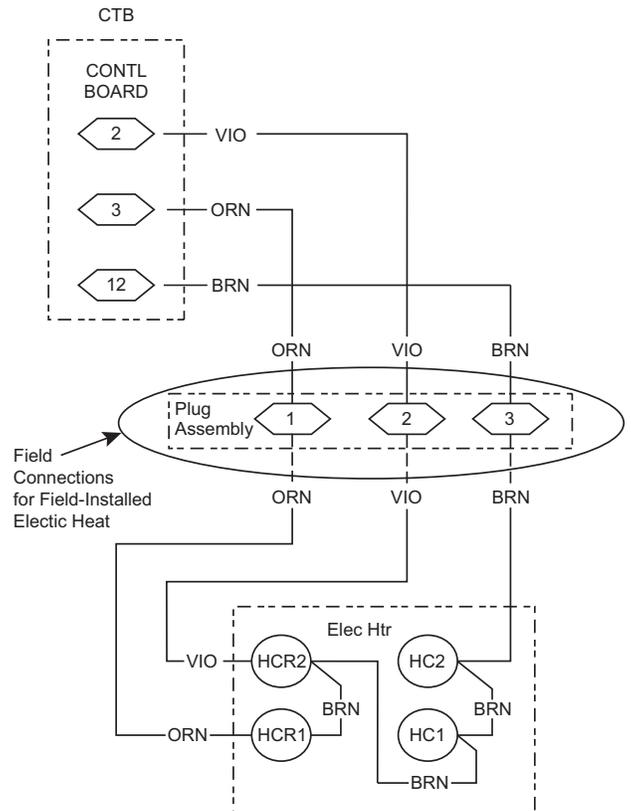
**Fig. 34 — Accessory Electric Heater Control Connections**
