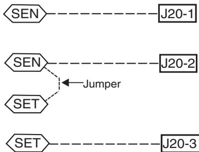
**Fig. 70 — RTU Open Controller T-56 Sensor Connections**
