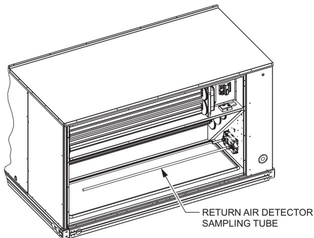
**Fig. 83 — Return Air Sampling Tube Location in Unit without Economizer**
