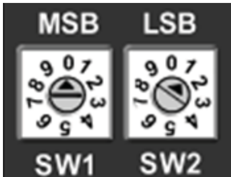
Fig. 70 - RTU Open Controller Address Switches
