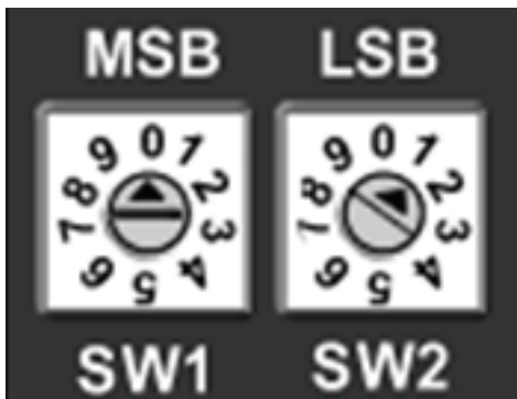
Fig. 69 - RTU Open Address Switches
