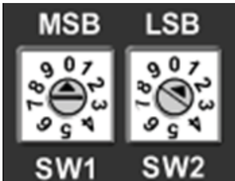
Fig. 71 - RTU Open Address Switches
