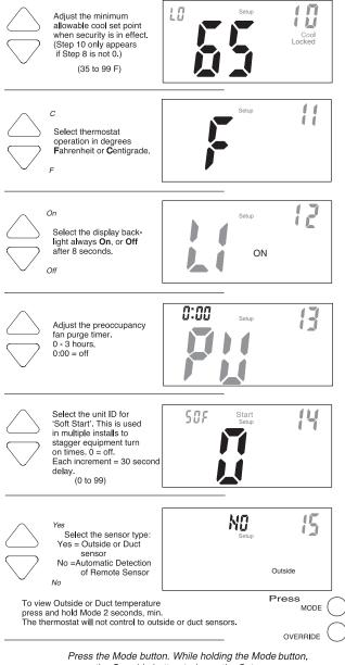
Press the Mode button. While holding the Mode button press the Override button to leave the Setup screens. If no buttons are pressed, the display will leave the set up screens after 30 seconds.
