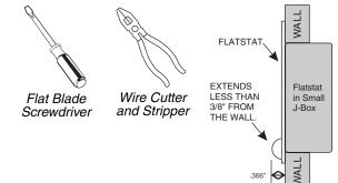
For best operation, install the thermostat in a junction box that is free from drafts that originate inside the wall.
