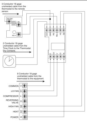
NOTE: H2 connection is not required for cooling only systems.
