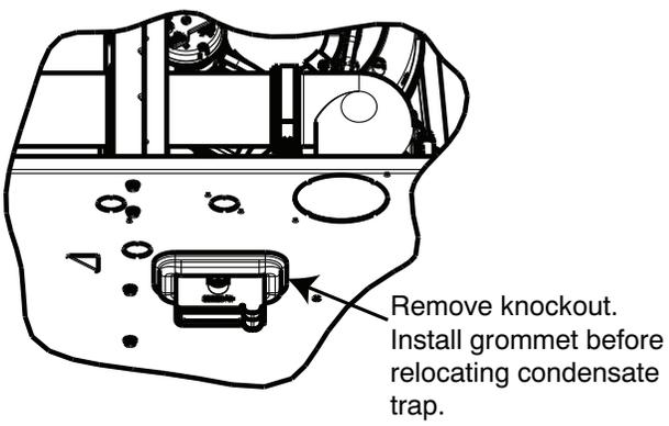
Fig. 17 - Horizontal Drain Trap Grommet
