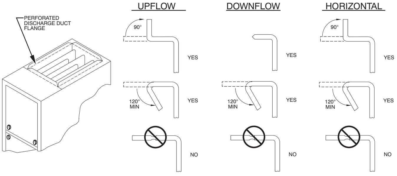
Fig. 21 - Duct Flanges
