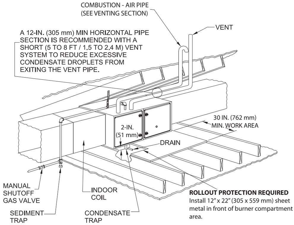
NOTE: FURNACE SHOWN AS DIRECT VENT APPLICATION. REFER TO THE VENTING SECTION FOR ALLOWABLE VENT CONFIGURATIONS
