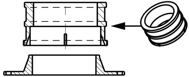
Attach gaskets to vent pipe and combustion air adapters.
