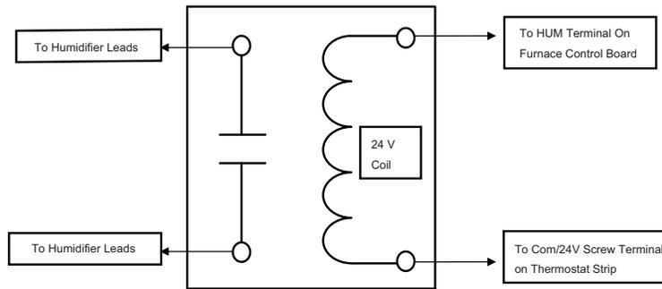
**Fig. 34 - Field-supplied Isolation Relay for Humidifiers with Internal Power Supply**
