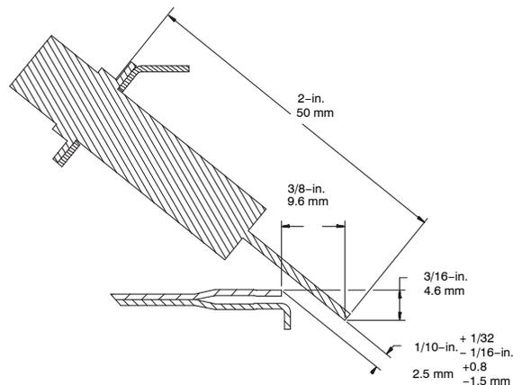
Fig. 63 - Igniter Position - Side View
