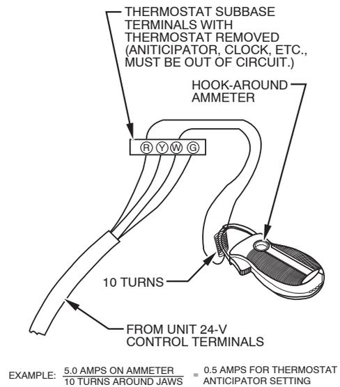
Fig. 59 - Amp. Draw Check with Ammeter
