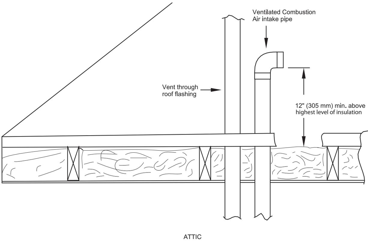
Fig. 54 - Vent Terminations for Ventilated Combustion Air
