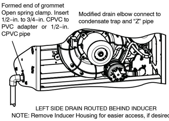
Fig. 18 - Drain Trap Connection and Routing
