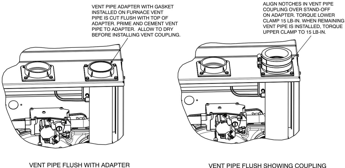
**Fig. 47 - Optional Vent Pipe Flush with Adaptor**
