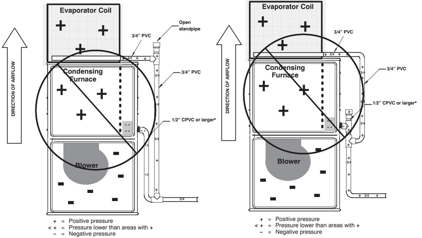
Fig. 13 - Example of Field Drain Attachment (Not Allowed)
