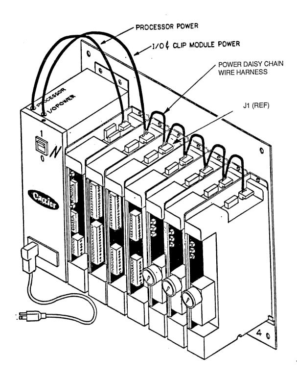
Figure 8 - Module Power Wiring
