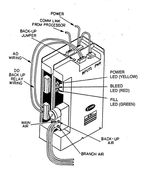
note For the purpose of illustrating output module to CLIP Module wiring, this figure shows an output module along with the CLIP Module.
