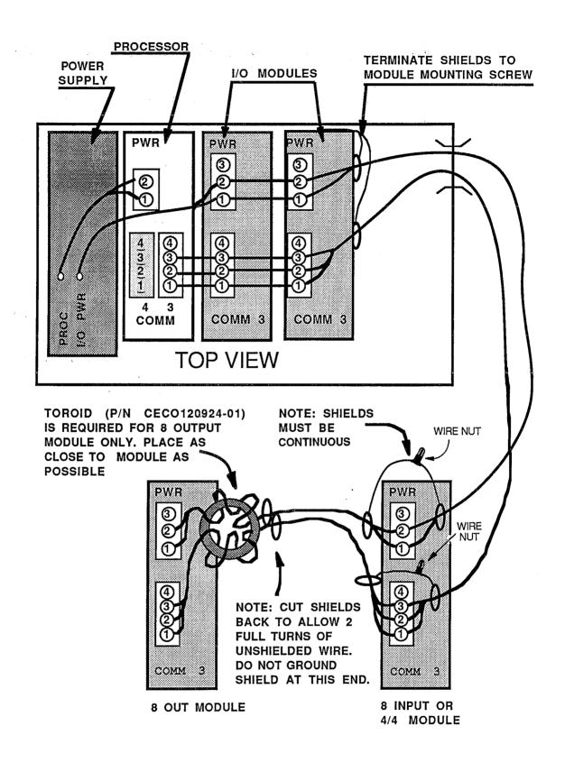
Figure 14 - Remote Module Power & Communication Wiring (Using the UT203 FID's Power Supply)
