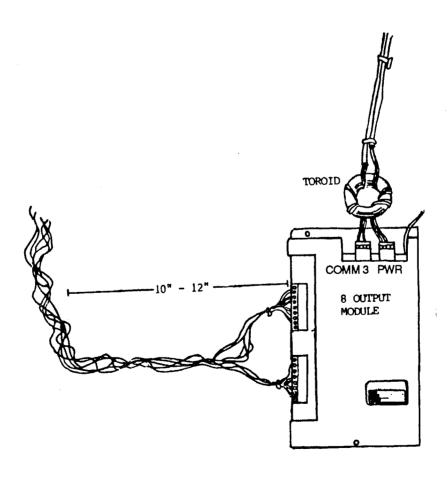
Figure 18 - Remote 8 Output Module Power & Communication Wiring
