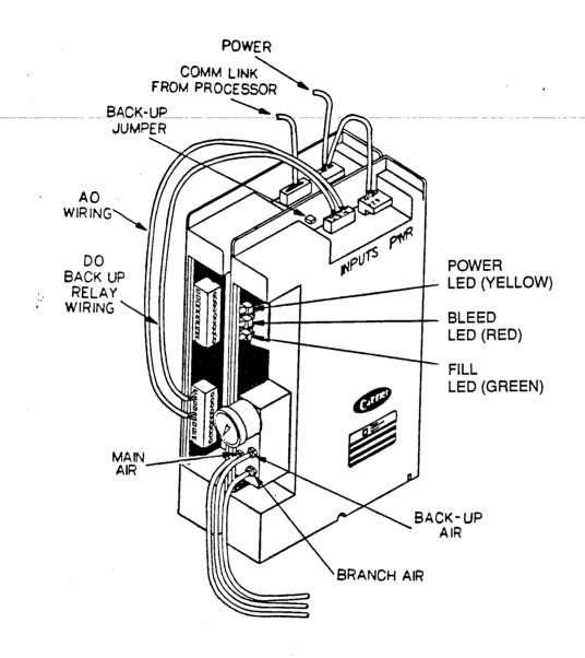
For the purpose of illustrating output module to CLIP Module wiring, this figure shows an output module along with the CLIP Module.
