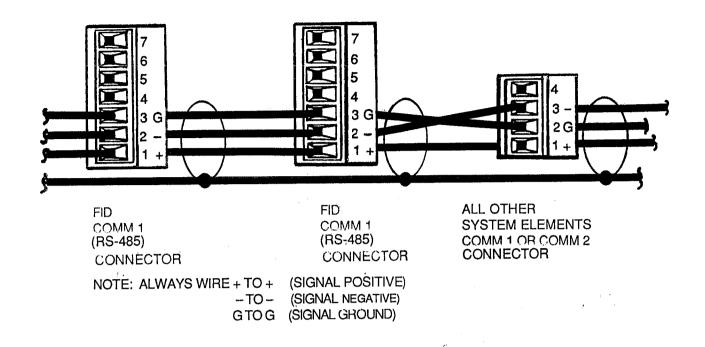
Figure 4 - CCN Communication Bus - UT203 FID Wiring
