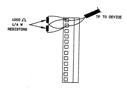
Figure 5 - Converting Analog Output to 2-10 Vdc
