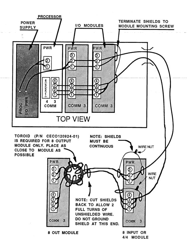
Figure 17 - Remote Module Communication & Power Wiring
