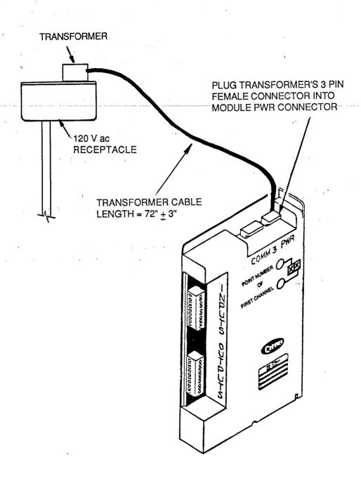
Figure 16 - Remote Module - Powered by a Local Power Supply
