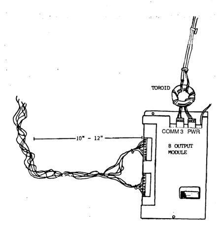
Figure 15 - Remote 8 Output Module Power and Communication Wiring
