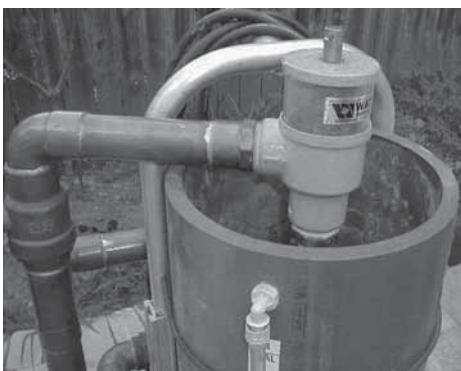
Figure 14a: Typical Cleanable Flush Cart Strainer (100 mesh [0.149mm])
