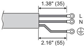
Attach a ring tongue terminal to the end of each wire of the power cable, communication cable and power cable for central controller.
