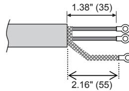
Length of stripped digital Input / Output communication wire
