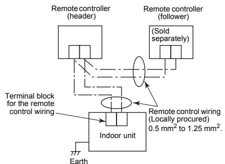
**To operate a group control of multiple indoor units by two remote controllers**
