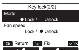
**1** Push the [ ]/[ ] button to select "5. Key lock" on the "Initial setting" screen, then push the " Set Set" [] button.
