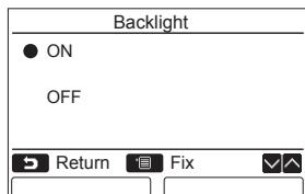
**1** Push the [ ]/[ ] button to select "4. Backlight" on the "Initial setting" screen, then push the " Set Set" [] button.
