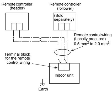
**To diverge from the header remote controller**
