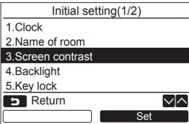
**1** Push the [ ^ ^ ] / [ v v ] button to select “3. Screen contrast” on the “Initial setting” screen, then push the “ Set Set” [F2] button.
