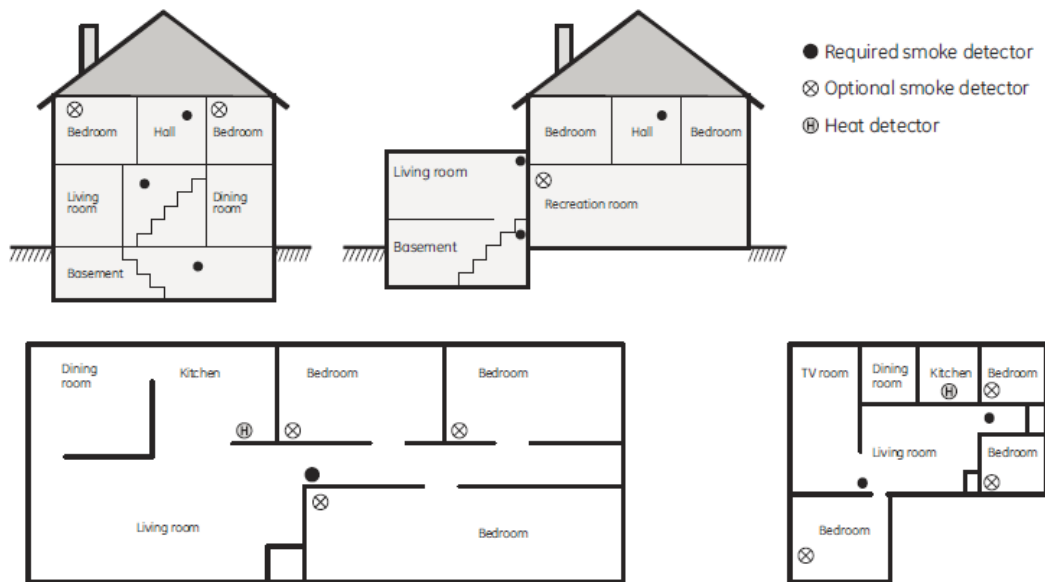
Fig. 3 - Smoke and Heat Detector Locations
