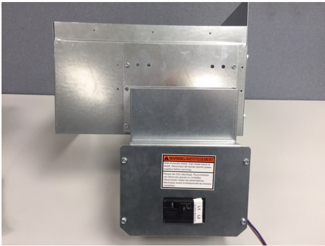
Fig. 7 — 10 Kw Heater Inserted in Collar with Top Plate Still in Place
