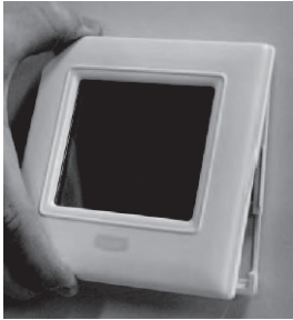
Fig. 11 - Attach Display to Backplate
