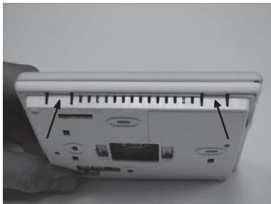
Fig. 5 - Press Tabs to Remove Backplate
