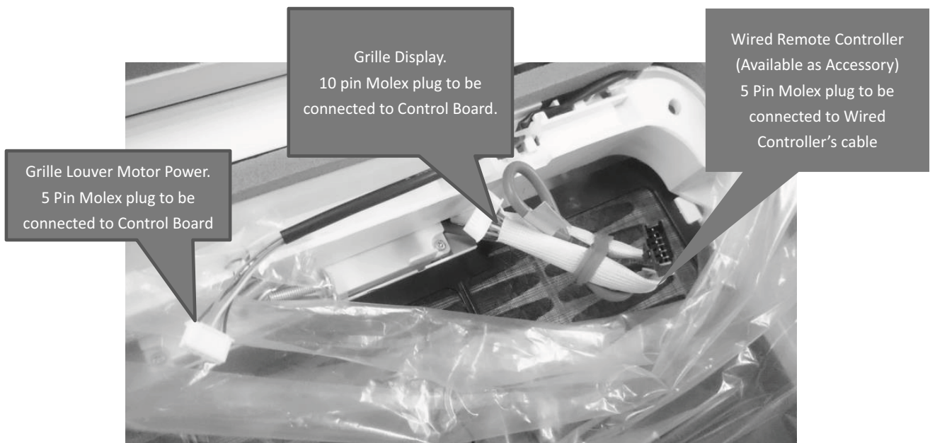
Fig. 29 – Panel Cassette Connections
