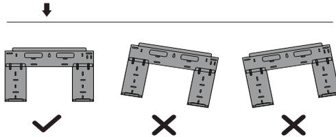
Fig. 8 – Mounting Plate Orientation
