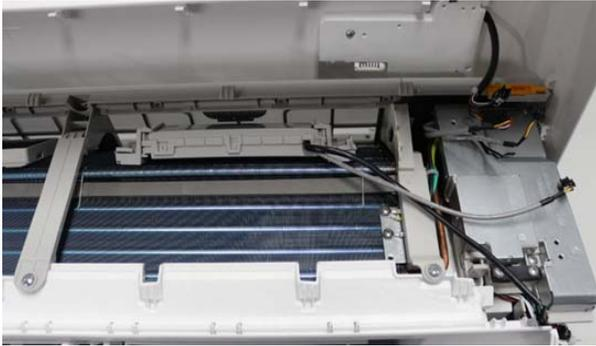
**Fig. 32 — Connect the multi-function board**
