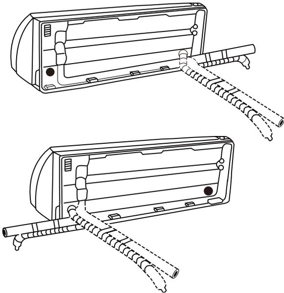
Fig. 11 – Piping Angle
