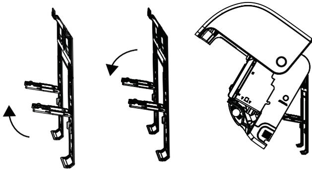
**Fig. 15 – Use Holder to Prop up the Unit**
