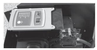
6. On 8 kW units, the main breaker is located inside the generator at the rear of the connection area.
