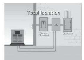
1. The generator will be backing up all electrical loads within the panel, so the amperage rating of the transfer switch must be equal to or greater than the amperage rating of the normal utility service.
