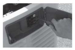
8. Remove the plastic plugs inside the main breaker access area to allow connection of the power leads to the circuit breaker.
