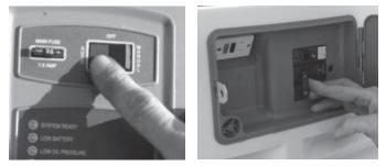
12. Switch the generator's main breaker ON and put the mode switch in AUTO.
