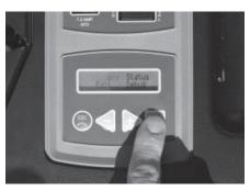
4. Press the left or right arrow key until 'Edit' is flashing and press enter.
