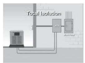
2. A service entrance rated transfer switch is installed between the service entrance and the main distribution panel. The service entrance rated switch becomes the main service so no service disconnect is needed. The existing main distribution panel becomes a sub-panel.
