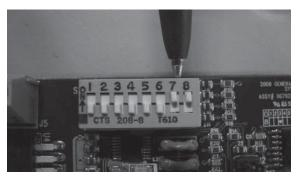
7. Locate the dip switches on the transfer switch control board and set them for the desired load shed delay as instructed in the transfer switch owner's manual.
