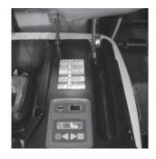
3. Remove the two screws securing the connection area cover, and remove the cover.
