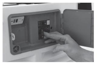
10. Switch the generator's main breaker ON. The generator is now ready for automatic operation.
