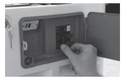
6. When finished checking the voltage, switch the generator's main circuit breaker OFF and put the mode switch in the OFF position to shut down the generator.
