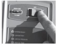
7. Put the generator's mode switch in MANUAL to start the engine.
