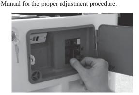
9. Switch the generator's main circuit breaker OFF and put the mode switch in the OFF position to shut down the generator.
