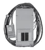
2. If the RTS Load Center transfer switch was purchased separately from the generator, the 5' seal-tite whip will need to be connected to the generator. To complete the wiring, run the <sup>3</sup>/<sub>4</sub>" conduit for the power leads and control wires from the external connection box to the generator.
