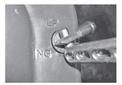
2. Take the plastic T-handle fuel selector in the poly bag supplied with the generator and locate the selector tab on the air box cover. Insert the pin end into the hole in the selector tab and pull outward to overcome spring pressure. Then twist clockwise 90 degrees and allow the selector to return in once aligned with the LP position.
