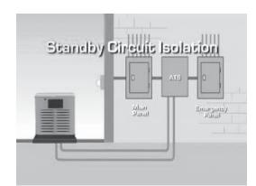
The generator powers only designated circuits that are grouped together and wired into a separate priority distribution panel. The transfer switch is installed between the main distribution panel and the priority panel. The amperage rating of the transfer switch must be equal to or greater than the highest amperage rating of the utility and generator breakers feeding the switch.
