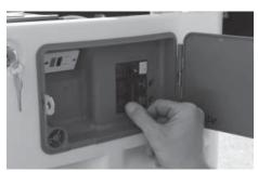
1. Switch the generator's main circuit breaker OFF and put the mode switch in the OFF position.
