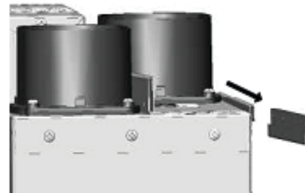
Fig. 9 - Slide ERV onto J-Hook
