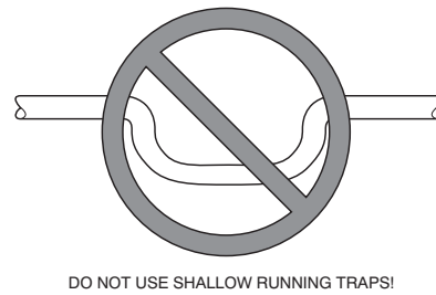
Fig. 21 - Insufficient Condensate Trap
